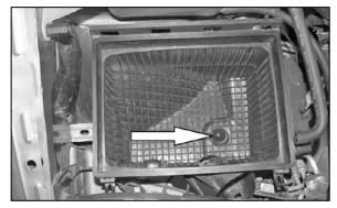
8. Remove the airbox mounting bolt shown.
