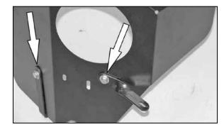
13. Install the Install the heat shield mounting bracket and twist bracket onto the heat shield as shown using the provided hardware.
