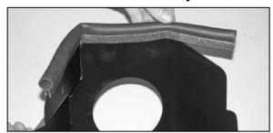
10. Install the provided edge trim onto the heat shield as shown.
