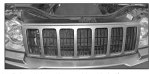
35. Reinstall the grill assembly with the factory retaining clips removed in step #5
