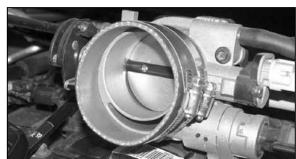
21. Install the silicone hose (08690) onto the throttle body and secure with the provided hose clamp.
