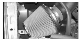
34. Install the air filter assembly onto the K&N® intake tube as shown and secure with the provided hose clamp.
