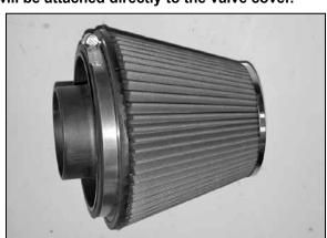
32. Install the filter adapter into the air filter as shown, secure with the provided hose clamp.
