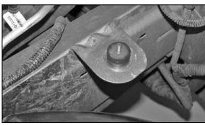
17. Using the two fender washers and one rubber washer, install the 6mm male/female rubber mounted stud onto the lower airbox mount as shown.
