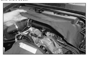
2. On 2008 and later model vehicles, pull up on the engine cover to dislodge it from the mounting grommets and then remove the engine cover from the vehicle.
