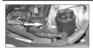
23. Remove the Lower rear A/C mounting bolt
