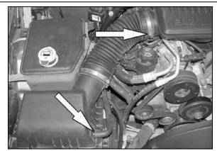
2a. Loosen the hose clamp, which secures the stock intake tube to the intake plenum, and disconnect the crankcase vent hose from the airbox lid.
