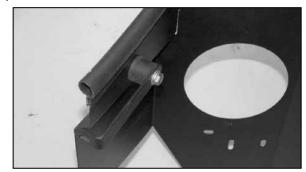
12. Install the bracket/rubber mounted stud assembly onto the heat shield as shown using the provided hardware.
