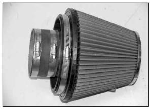
33. Install the silicone (08630) onto the air filter assembly and secure with the provided hose clamp.
