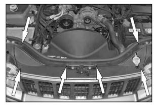
5. Using a small screwdriver, release the center holding pins in the six grill retaining clips shown.
