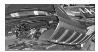
6. Remove the six grill retaining clips from the grill, then tilt the grill forward and lift to remove from the vehicle.
