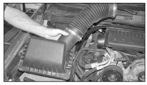
3. Unclip the upper airbox retaining clips and remove the upper airbox and intake tube assembly as shown
