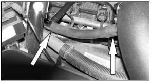
31.Install the supplied silicone hose onto the crankcase vent "T" and connect the other end onto the K&N® intake tube as shown.
