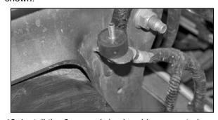
18. Install the 6mm male/male rubber mounted stud onto the upper airbox mount as shown.
