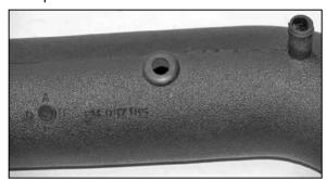
26. Install the supplied rubber grommet into the K&N® intake tube as shown.
