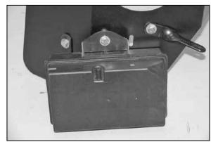
15. Using the provided spacer, install the vacuum reservoir onto the heat shield as shown.
