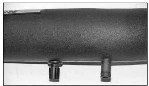
28. Install the air temperature sensor into the K&N® intake tube as shown.
