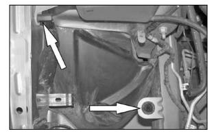
16. Remove the coolant reservoir-retaining nut and airbox mounting grommet shown.
