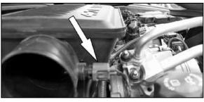
20a. Disconnect the air temperature electrical connection.
