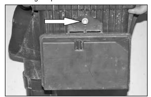
14. Remove the bolt which secures the vacuum reservoir to the airbox and then remove the reservoir from the airbox.
