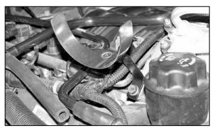
24. Install the tube mounting bracket assembly onto the A/C compressor and secure with the factory-mounting bolt removed in step #23.
