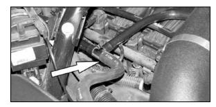
30. Remove the factory crankcase vent hose from the "T" fitting shown.
