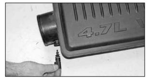
25. Rotate the air temperature sensor counter clockwise and remove the sensor from the stock intake plenum as shown.
