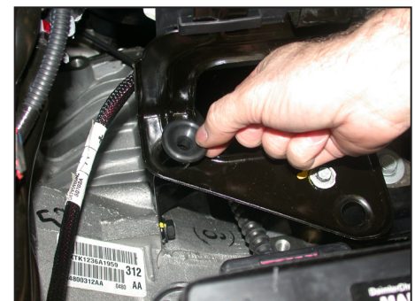
7. Remove the two airbox retaining grommets from mounting tray as shown.
