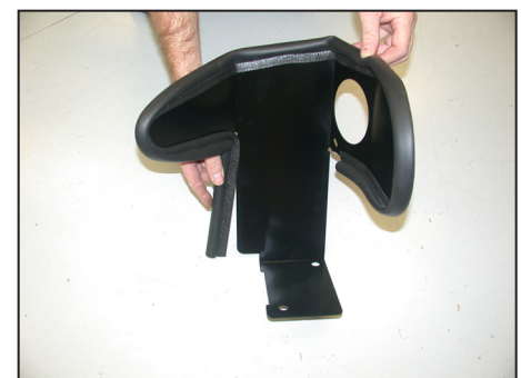
9. Install the long edge trim onto the heat shield as shown. NOTE: Some trimming of the edge trim may be necessary.
