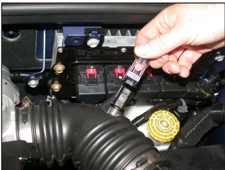
2. Disconnect the air temp. electrical sensor as shown.
