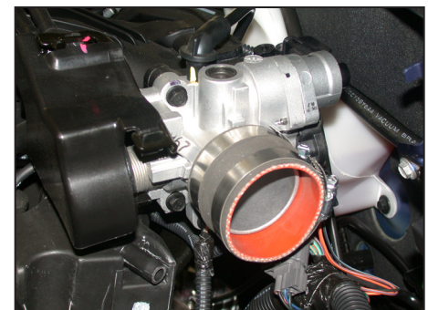
8. Install the silicone hose (08405) onto the throttle body and secure with the provided hose clamp as shown.
