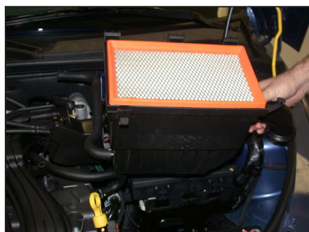
6. Pull up firmly on the airbox base to dislodge it from the retaining grommets and then remove the airbox from the vehicle. NOTE: K&N Engineering, Inc., recommends that customers do not discard factory air intake.
