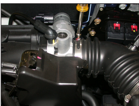
3. Loosen the hose clamp, which secures the intake tube to the throttle body.
