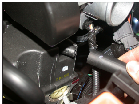
5. Disconnect the crankcase vent hose from the valve cover as shown.
