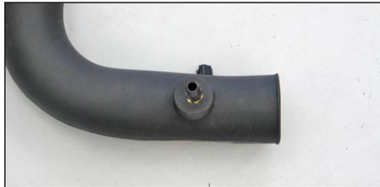
17. Install the supplied 1/4" npt vent fitting into the threaded boss in the K&N® intake tube as shown.
