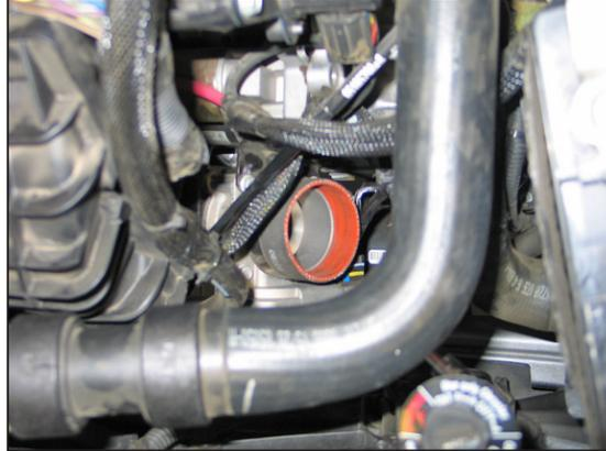
13. Install the silicone hose (08108) onto throttle body and secure with the provided hose clamp.
