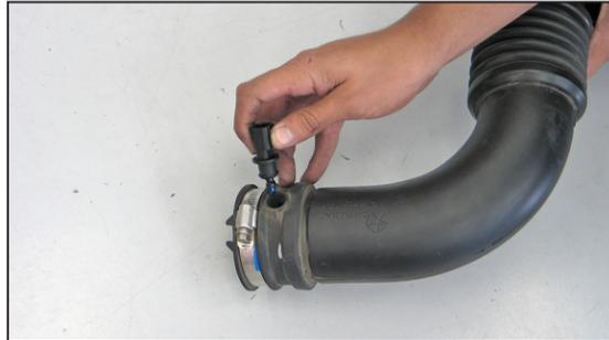
15. Remove the air temperature sensor from the factory intake tube as shown.
