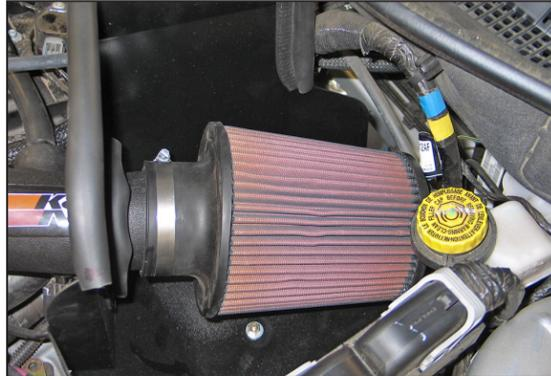
29. Install the K&N® air filter and secure with the provided hose clamp.
