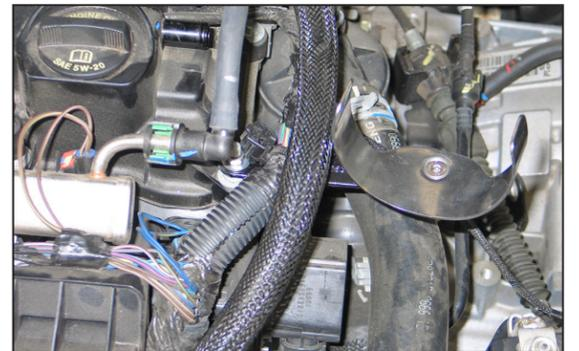
21. Install the tube mounting bracket assembly onto the valve cover stud and secure with the provided hardware.
