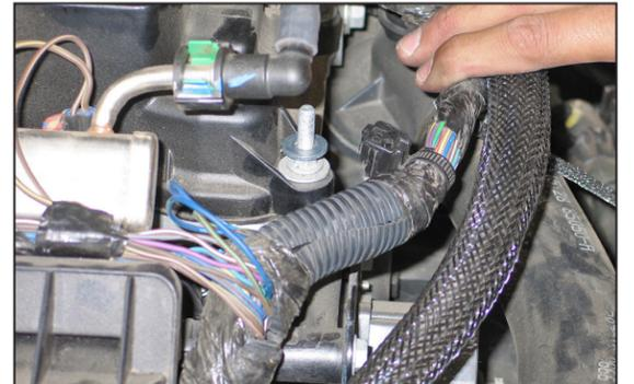
20. Place one washer onto the valve cover stud as shown.
