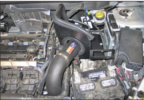
26. Install the K&N® intake tube into the silicone hose and align onto the saddle clamp. Then secure with the provided hose clamps. Tighten bolts in #21.
