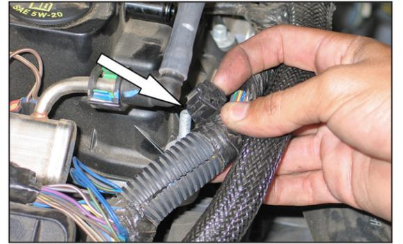
19. Unhook the wiring harness from the corner valve cover bolt as shown.
