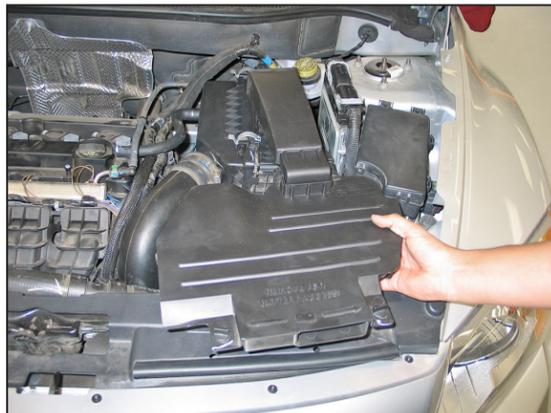
4. Remove the fresh air duct from the stock air filter housing and radiator core support.
