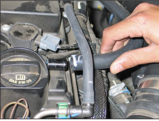
7. Disconnect the crankcase vent hose from valve cover.
