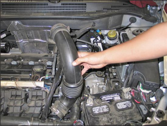
10. Remove the stock intake tube from the vehicle.
