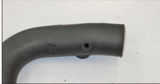
14. Install the supplied grommet into the intake tube as shown.
