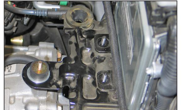
22. Install rubber mounted stud using the large fender washers provided.
