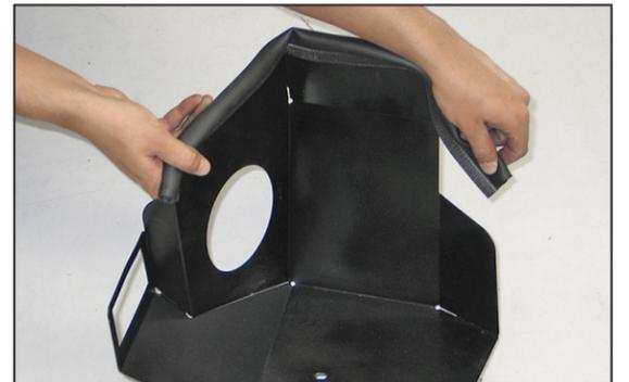
23. Install the long edge trim along the top of the heat shield as shown.
