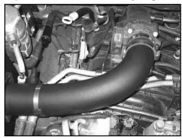
23. Install the K&N<sup>®</sup> intake tube into the into the silicone hose on the throttle body and position so the tube aligns with the saddle clamp. Secure the tube with the provided hose clamps.
