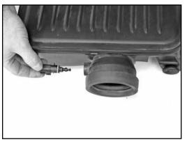
20. Twist the air temperature sensor counter clockwise and remove it from the stock intake plenum.
