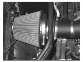
28. Install the air filter assembly onto the K&N<sup>®</sup> intake tube and secure with the provided hose clamp.
