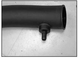
NOTE: NPT fitting has tapered threads and only designed to be installed until hand tight, then tighten one rotation or when the fitting becomes difficult to return.
