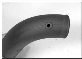
19. Install the provided grommet into the  $K\&N^{\textcircled{R}}$  intake tube as shown.
