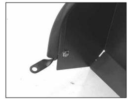
9. Install the twist bracket (070702) onto the heat shield with the provided hardware as shown.
