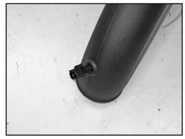
22. Install the air temperature sensor into the grommet installed into the K&N<sup>®</sup> intake tube in step #19.
