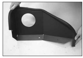
7. Install the provided edge trim onto the heat shield as shown. NOTE: Some trimming of the edge trim may be
