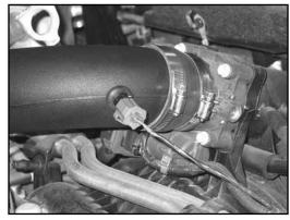
24. Reconnect the air temperature sensor electrical connection.
