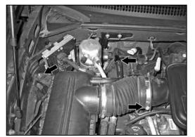
2. Loosen the hose clamp at the intake plenum
