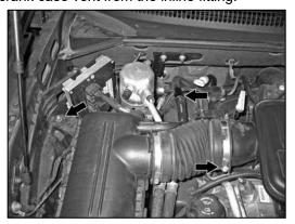
3. Disconnect the stock intake tube from the intake plenum. Lift to remove to remove the air box assembly from the vehicle as shown. 5. Lift to dislodge the intake plenum from it's mounting grommets and remove the intake plenum from the vehicle as shown.
