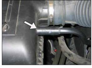
4. Disconnect the crank case vent hose from the air box.
