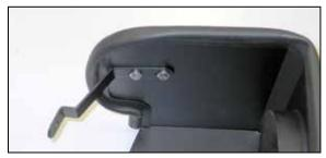
15. Install the heat shield mounting bracket (083127A) onto the heat shield using the provided hardware.
