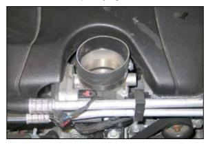
20. Install the provided silicone hose (08698) onto the throttle body and secure with the provided hose clamp.
