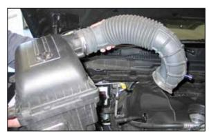
5. Disconnect the factory intake hose from the throttle body, then lift up the air box assembly and remove from the vehicle.
