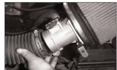
13. Attach the intake tube to the mass air sensor.
