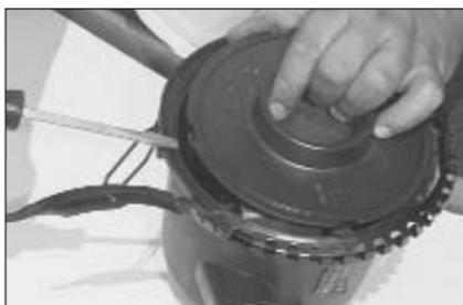
8. Using a flat blade screwdriver, depress tabs on cover to remove mass air sensor.
