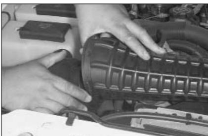
5. Detach the intake tube from the airbox.
