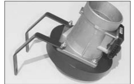
12. Using the hardware provided, assemble the mass air adapter, gasket and brackets as shown in illustration above.
