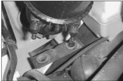
6. Pull firmly up on airbox to release airbox from grommets on lower airbox support bracket assembly.
