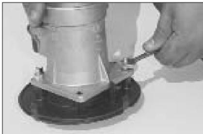
9. Loosen and remove the nuts from the mass air sensor.
