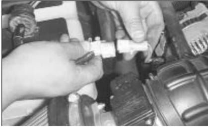
18. Reconnect the secondary mass air sensor electrical connection.
