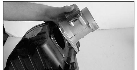
8. Loosen and remove the four bolts that secure the mass air sensor, then remove the mass air sensor as shown.
