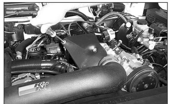
27. Re-install the throttle linkage cover as shown.
