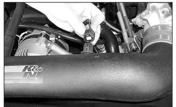
25. Reconnect the air temp sensor electrical connections as shown.
