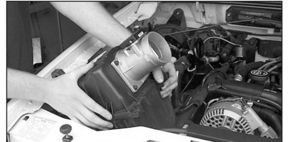
7. Using a screwdriver, pry up on the bottom of the air cleaner assembly to release the air cleaner from the factory grommets, then remove the air cleaner assembly as shown.
