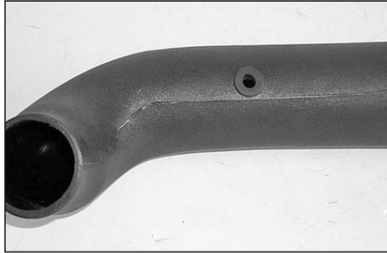
17. Install the provided grommet onto the K&N intake tube as shown.
