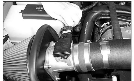
26. Reconnect the mass air sensor electrical connection as shown.
