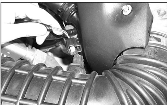
3. On models that come equipped with an air temp sensor, disconnect electrical connection.
