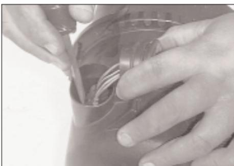
13. Pull rubber boot back away from airbox. Depress tab with screwdriver as shown to release electrical connection.
