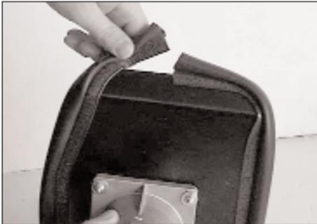
17. Apply the trim seal to the heat shield assembly as shown.
