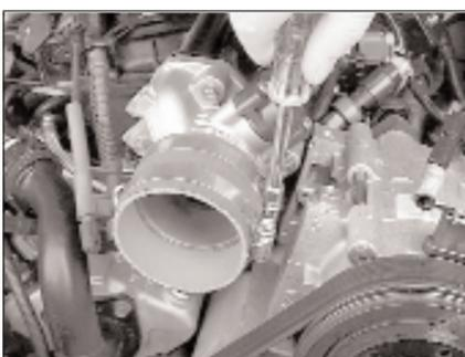
19. Install the silicone hose and hose clamps onto the throttle body as shown.
