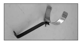
6. On vehicles that come equipped with A/C, assemble the saddle bracket onto bracket (07164A) as shown.
