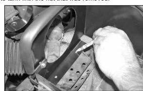
12. Install the heat shield onto the vehicle then line up the fresh air duct to the heat shield and mark the two holes with a marker, then remove heat shield from vehicle.
