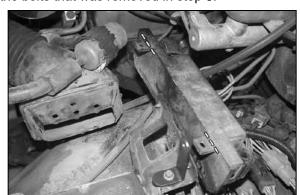
10a. On vehicles that come with a relay mounting bracket cut the two tabs off for heat shield clearance as shown.
