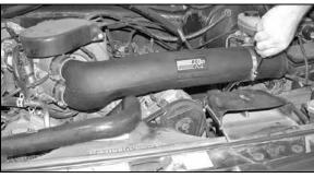
15. Install the new K&N® intake tube onto the throttle body, then secure the intake tube to the saddle bracket as shown.
