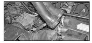
3. Loosen the two hose clamps at the airbox then remove the two intake tubes from the air box as shown.
