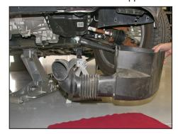
12. On vehicles equipped with an air box cover, lower the cover and remove it from the vehicle.
