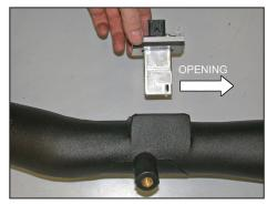
22. Install the mass air sensor assembly into the  $K\&N^{\circledast}$  intake tube.
