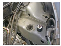
25. Install the rubber mounted stud into the threaded hole in the frame rail as shown.
