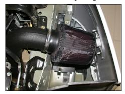
29. Install the air filter onto the K&N<sup>®</sup> intake tube and secure with the provide hose clamp.
