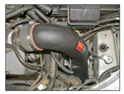
26. Install the K&N<sup>®</sup> intake tube assembly into the silicone hose at the throttle body and onto the rubber mounted stud, then secure with the provided hardware.
