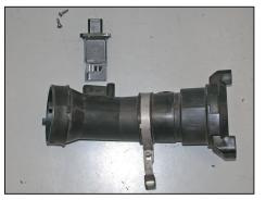
19. Remove the mass air sensor from the factory mass air sensor housing using the Torx wrench provided.
