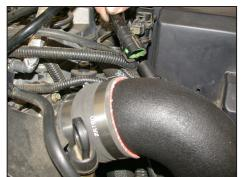
27. Reconnect the crank case vent hose to the fitting installed into the  $K\&N^{\otimes}$  intake tube in step #18.
