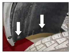
10. After jacking up the car and placing on suitable jack stands and chocking the rear wheels, remove the two bolts which secure the air box on equipped vehicle's or the one bolt on splash shield equipped vehicle's to the inner finder well.
