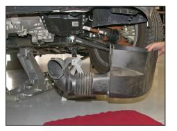
30. On vehicle's that were equipped with an air box cover, reinstall and secure with the bolts that were removed in step #11.
