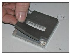
20. Apply the provided gasket onto the K&N<sup>®</sup> mass air adapter as shown.
