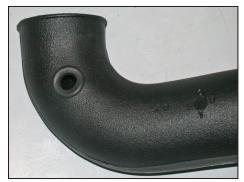
17. Install the provided grommet into the K&N $^{\mbox{\tiny \$}}$  intake tube as shown.
