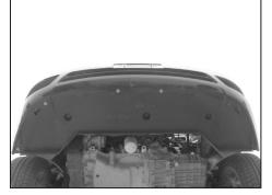
30a. On vehicle's that were equipped with the splash shield, reinstall with the bolts removed in step #10a.
