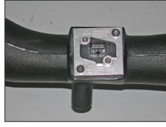
23. Secure the mass air sensor assembly into the K&N^ $\ensuremath{\mathbb{S}}$  intake with the provided hardware as shown.
