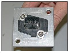
21. Using the factory mass air bolts, install the mass air sensor into the K&N $^{\mbox{\tiny ®}}$  mass air adapter as shown.
