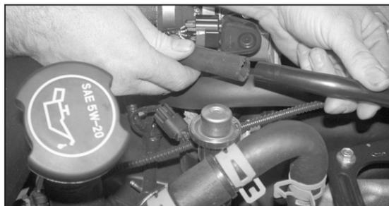
16. Cut the factory crank case vent tube one inch from the end, then attach the supplied silicone vent hose to the K&N® intake tube and factory vent tube as shown.
