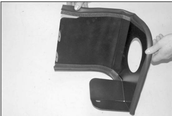
9. Install the edge trim seal onto the heat shield as shown.
