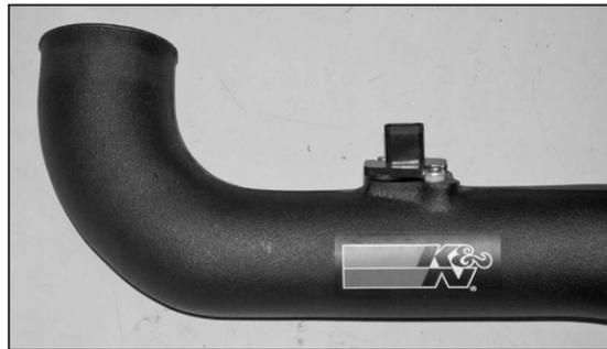
14. Install the mass air sensor into the K&N® intake tube and secure with the factory screws and spacers provided.
