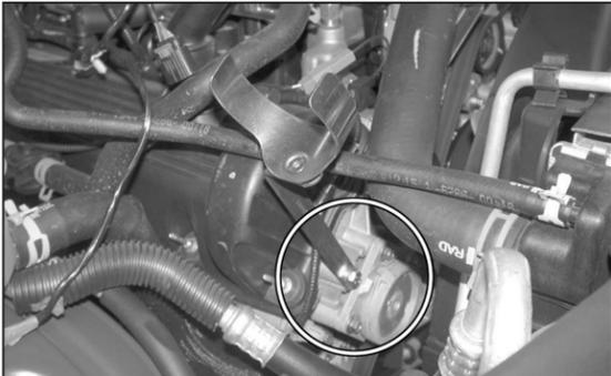
8. Using the 8mm bolt washers supplied, attach the tube mounting bracket assembly to the front of the engine at the threaded boss above the belt tensioner as shown.
