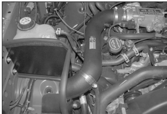
15. Install the K&N® intake into the silicone hose at the throttle body and onto the saddle clamp, then secure with the provided hose clamp.
