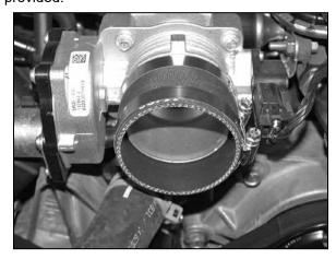
16. Install the silicone hose (08434) onto the throttle body with the provided hose clamps as shown.
