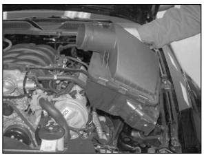
6. Remove the airbox assembly as shown.
