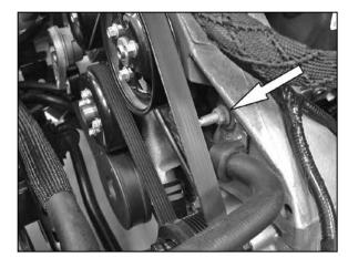
7. Remove the power steering pump bracketretaining nut shown.
