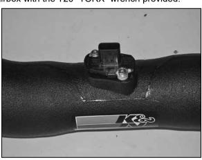
15. Install the mass air sensor into the K&N® intake tube with the mounting screws and two spacers provided.
