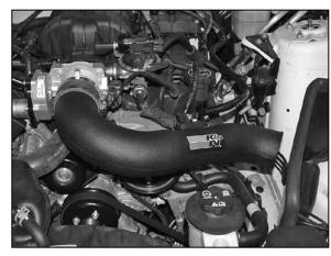
17. Install the K&N® intake tube into the silicone hose at the throttle body and onto the tube-mounting bracket installed in step #8, secure with provided hardware.
