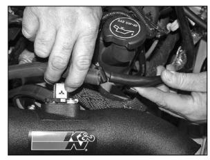
19. Install the provided crankcase vent hose onto the K&N® intake tube and factory vent hose as shown.
