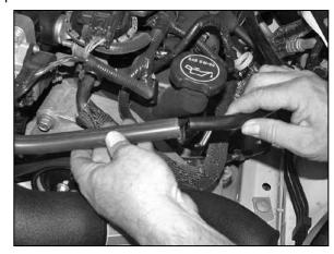
18. Using a razor blade cut the crankcase vent tube 6" from the end as shown.
