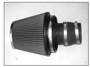
21. Install the silicone hose (08724) onto the air filter assembly and secure with the provided hose clamp as shown.
