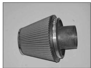
20. Install the air filter onto the filter adapter and secure with the provided hose clamp as shown.
