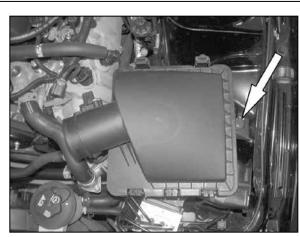
5. Remove the airbox mounting bolt shown.
