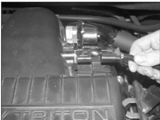
2. Disconnect mass air sensor electrical connection.
