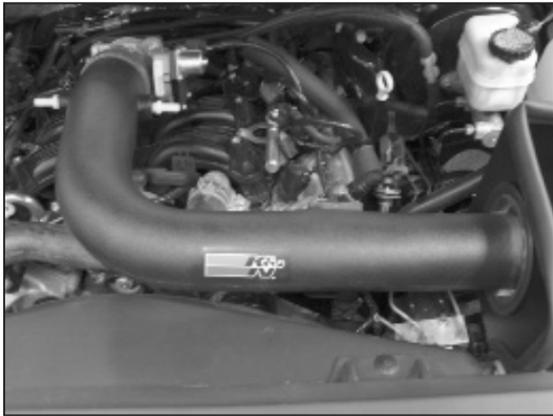
31. Install the K&N® intake tube onto the throttle body and position so that it lines up with the tube mounting bracket installed in step #29. Secure the intake tube with the provided bolt and hose clamp.
