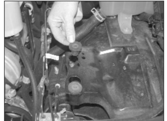
18. Install the provided nut inserts into the air box mounting holes as shown.
