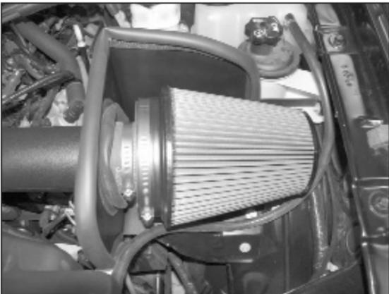
40. Install the K&N® Air filter assembly onto the K&N® intake tube as shown and secure with the provided hose clamp.
