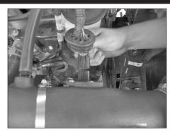
27. Reconnect the secondary mass air sensor electrical connection and then reconnect the mass air sensor primary electrical connection.
