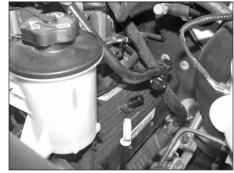
2. Rotate the crank case vent hose locking ring and pull the crank case vent hose off of the valve cover.
