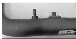
18. Install the provided 1/4" npt fitting into the K&N® intake tube as shown.
