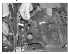
9. Install the provided nut inserts into the air box mounting holes as shown.
