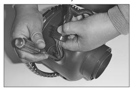
12. Slide the rubber grommet back and disconnect the primary mass air sensor electrical connection, using a flat blade screwdriver.
