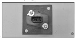
16. Install the mass air sensor into the adapter using the factory screws.
