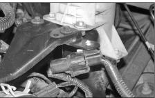
4. Unhook the secondary mass air sensor electrical connection from the power steering reservoir bracket, then unlock the electrical connection locking tabs and separate the electrical connection
