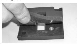
15. Remove the backing paper and install the mass air sensor adapter gasket as shown.
