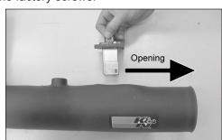
17. Install the mass air sensor assembly into the  $K\&N^{\circledcirc}$  intake tube and secure with the provided hardware.
