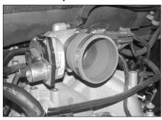
19. Install silicone hose (08724) onto the throttle body with the provided hose clamp as shown.
