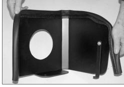
7. Install the edge trim onto the heatshield as
