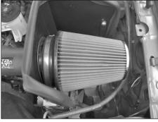
26. Install the filter assembly onto the K&N® intake tube and secure with the provided hose clamp. NOTE: Drycharger® air filter wrap; part # RF-1041DK is available to purchase separately. To learn more about Drycharger® filter wraps or look up color availability please visit http://www.knfilters.com®.
