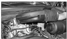
3. Loosen the stock intake tube hose clamps, and remove the intake tube from vehicle.
