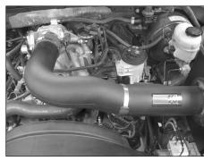
22. Install the K&N® intake tube into the silicone hose at the throttle body and onto the tube mounting bracket assembly. Secure with the provided hose clamps.
