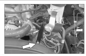
21. Install the tube mounting bracket assembly onto the 8mm stud protruding from the engine with the nut and washer provided.
