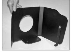
6. Install "L" bracket (070026) onto the heatshield with the hardware provided as snown.
