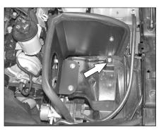
10. Install the heatshield as shown and secure with the provided hardware.
