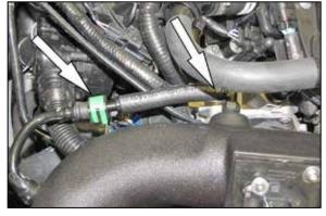
23. Install the EVAP hose assembly into the factory quick disconnect fitting and then onto the 90° fitting install into the K&N<sup>®</sup> intake tube as shown.
