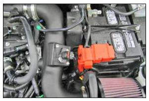
25. Connect the mass air sensor electrical connection as shown.
