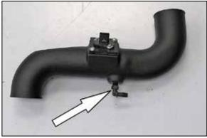
20. Install the 90° vent fitting into the K&N $^{\circ}$  intake tube as shown.
