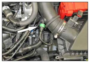
4. On vehicles with a single EVAP line, release the green locking tab and then disconnect the EVAP vent line from the factory intake tube.
