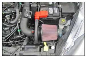
24. Install the K&N<sup>®</sup> air filter onto the intake tube and secure with the provided hose clamp. NOTE: Drycharger<sup>®</sup> air filter wrap; part # RX-4990DK is available to purchase separately. To learn more about Drycharger<sup>®</sup> filter wraps or look up color availability please visit http://www.knfilters.com<sup>®</sup>.
