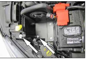
12. Secure the heat shield mounting bracket (064317) to the heat shield and core support as shown using the provided hardware.
