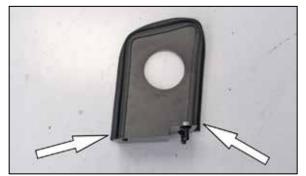
9.Install the provided "Top Bulb" edge trim around the outside of the heat shield as shown. **NOTE: Some trimming of the edge trim will be necessary.**
