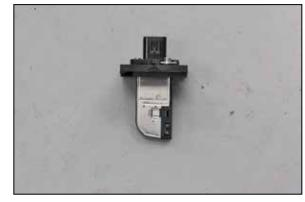
18. Install the mass air sensor into the K&N<sup>®</sup> adapter and secure with the provided hardware.
