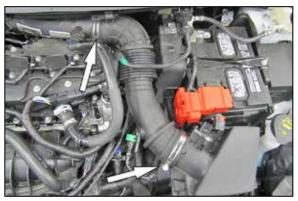
5. Loosen the hose clamps securing the factory intake tube to the turbo inlet pipe and to the factory air filter housing. Remove the factory intake tube from the vehicle.
