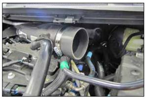
15. Install the provided coupling hose (08440) onto the turbo inlet pipe and secure with the provided hose clamp.
