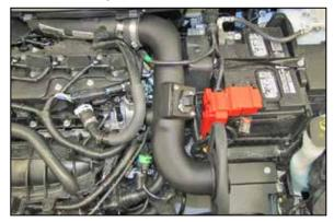
11. Install the heat shield into the vehicle so that the two mounting posts engage the air box mounting grommets.
