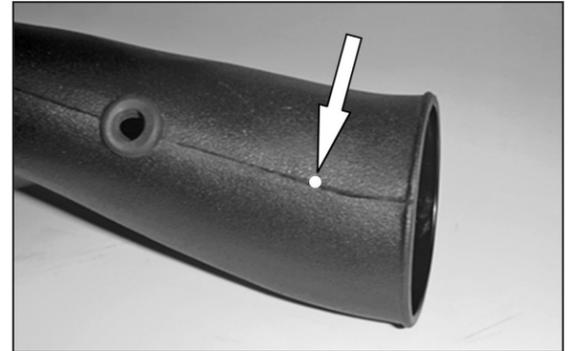
22. On models equipped with a fuel pressure regulator vacuum line, drill out the drill point in the K&N® intake tube using a 3/4" drill bit.
