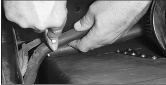
58. Cut the air injection vent hose as shown.
