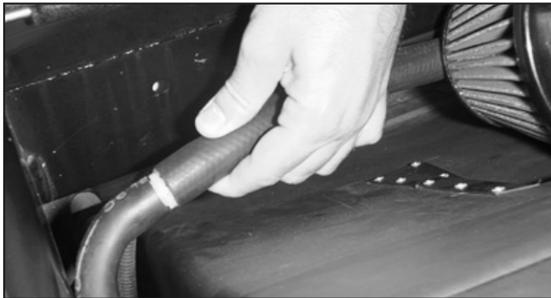
59. Attach the air injection hose to the hose mender.
