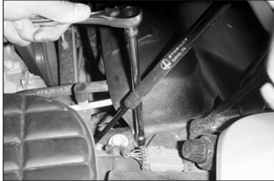
37. Loosen and remove the four bolts that retain the upper radiator cover.
