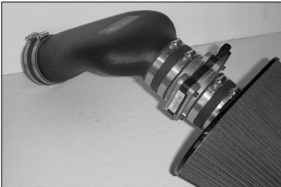
31. Assemble the intake tube and Air filter element assemblies.
