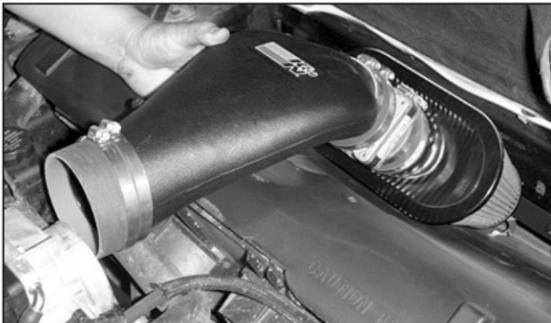
32. Install the K&N® intake assembly.
