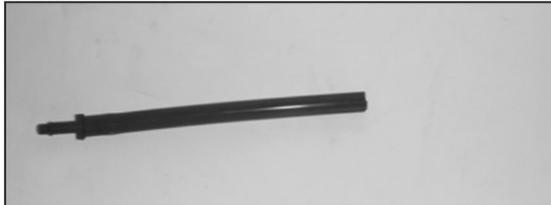
61. On models equipped with a fuel pressure regulator vacuum line, insert the OE vent into the 1/8" ID vent hose provided.
