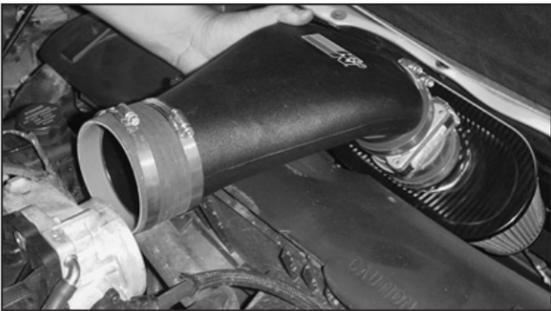
56. Reinstall the K&N® intake assembly then adjust the radiator cover for best fit under the intake tube, then tighten the 4 retaining bolts.
