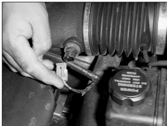
3. Disconnect the air temperature sensor electrical connection.
