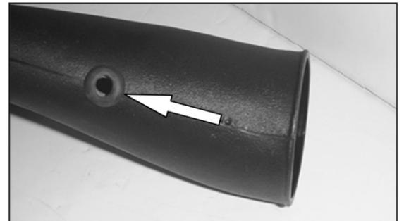
21. Insert the 1/2" ID grommet into the hole in the K&N® intake tube.
