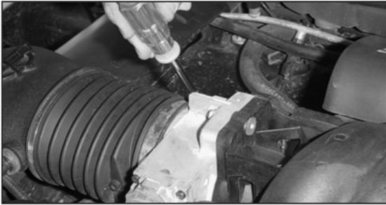
9. Loosen the hose clamp on the intake hose at the throttle body.
