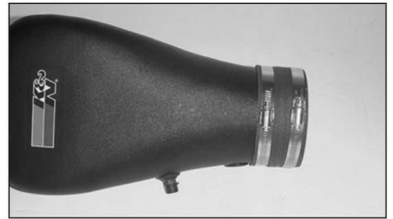
27. Install the 4" ID silicone hose onto the K&N® intake tube.
