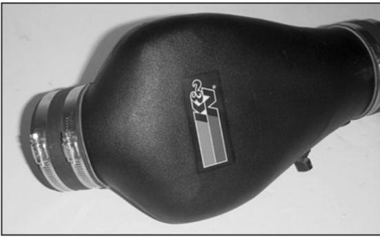
28. Install a 3.5" ID silicone hose (08630) onto the K&N® intake tube.
