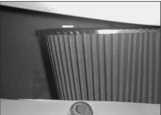
34. Using the top of the Air filter element as a guide, mark the lower radiator cover a minimum of 1/2" above the filter.
