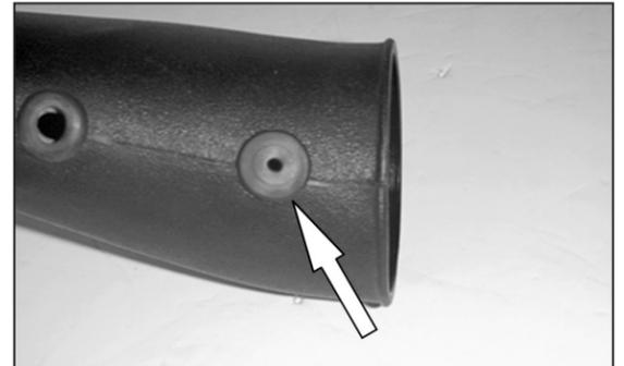
23. On models equipped with a fuel pressure regulator vacuum line, insert the 3/16" ID grommet into the hole drilled in the previous step.
