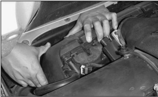
10. Pull the airbox towards the engine to release it from its mounting grommets.
