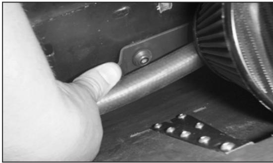
57. Install the angled bracket onto the original airbox mounting points.
