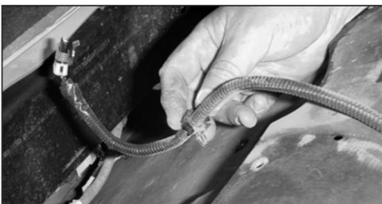
12. Detach the wiring harness retaining clip from the lower radiator cover.
