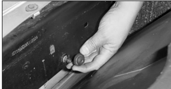
17. Remove the two grommets from the airbox mounting points.
