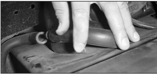
7. Disconnect the air injection vent hose.
