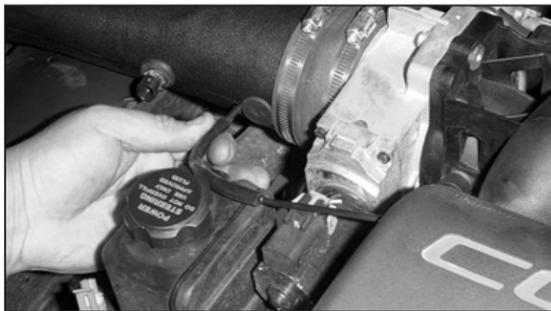
62. On models equipped with a fuel pressure regulator vacuum line, attach the 1/8" ID vent hose to the vacuum tube and insert the hose mender into the grommet.
