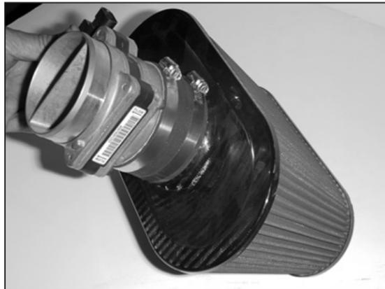
19. Install the mass air sensor into the silicone hose with the arrow on the mass air sensor pointing away from the Air filter element.
