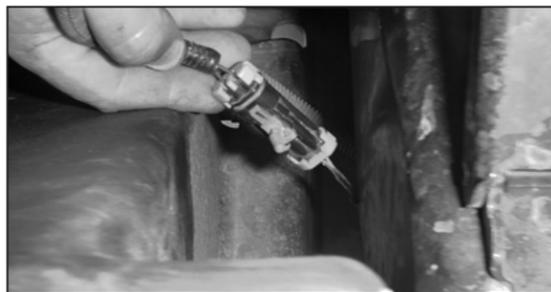
41. Detach the courtesy lamp wiring harness from the lower radiator cover.
