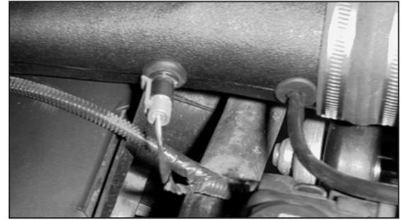
64. Reconnect the air temperature sensor electrical connection.
