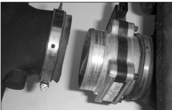
13. Loosen the hose clamp and detach the stock intake tube from the mass air sensor.
