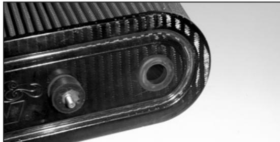
20. Install the 5/8" ID grommet and the rubber mounted stud into the top plate of the Air filter element.
