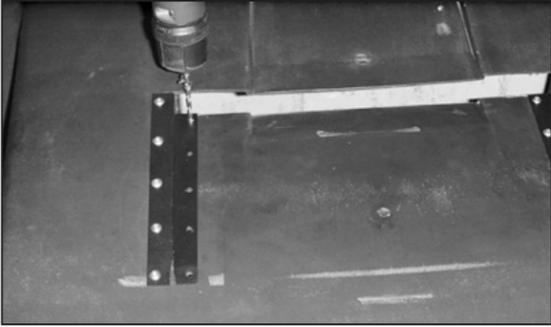
50. Drill out the five inner holes of each bracket.
