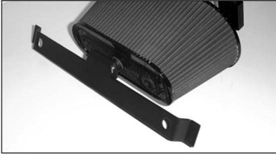
29. Attach the angled bracket to the rubber mounted stud using the provided hardware. **Note: Do not tighten completely at this time.**
