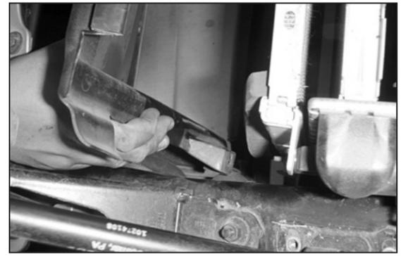
42. Pull firmly to release the radiator cover from its retaining clips.
