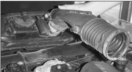
11. Detach the intake hose from the throttle body and remove the entire air intake assembly.
