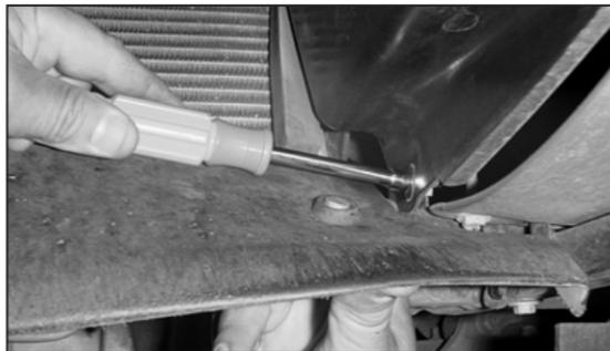
40. Loosen and remove the two bolts that retain the lower radiator cover to its mounting brackets.
