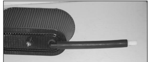
26. Insert the 90 degree vent into the grommet in the top plate of the filter.
