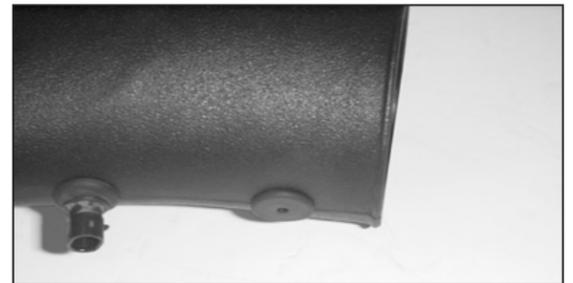
24. Insert the air temperature sensor into the 1/2" ID grommet.
