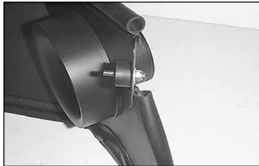
18. Attach a rubber mounted stud to the heat shield using the hardware provided. NOTE: Do not tighten completely at this time.
