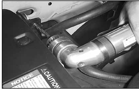
17. Using \frac{1}{4} " drill bit, drill out location marked in the previous step.
