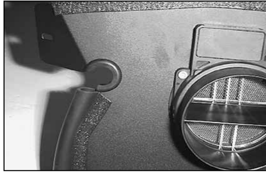
14. Install the grommet onto the heat shield.
