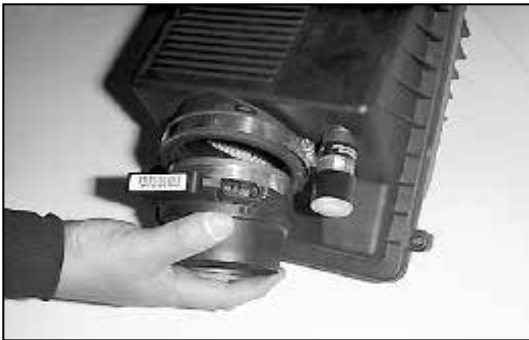
9. Loosen the hose clamp and remove the mass air sensor from the airbox.
