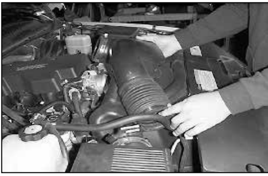
7. Detach the intake tube from the throttle body and remove the intake assembly.
