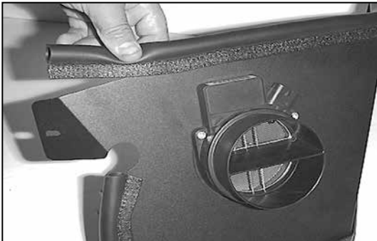
11. Install the trim seal onto the heat shield as shown. NOTE: Some cutting and trimming may be necessary to achieve best fit.
