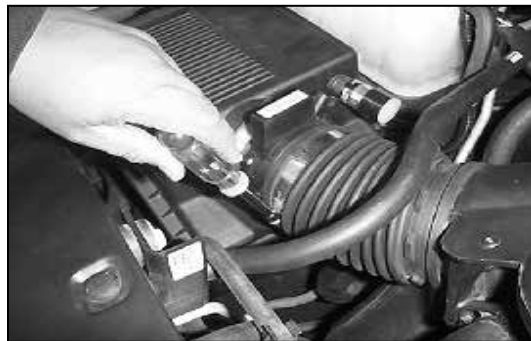
3. Loosen the hose clamp on the intake hose at the mass air sensor.
