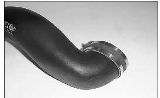
23. Install the 4"ID silicone hose onto the intake tube. NOTE: Do not tighten the hose clamps at this time.
