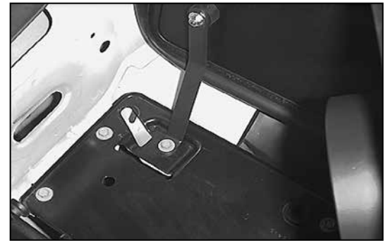
21. Secure the bracket to the airbox mounting tray using the bolt removed in step 19. NOTE: Do not tighten completely at this time.
