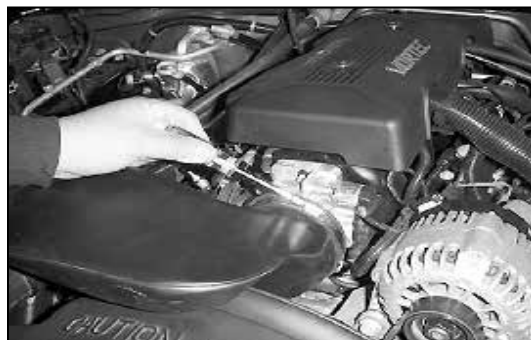
4. Loosen the hose clamp on the intake tube at the throttle body.
