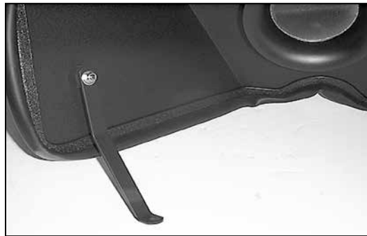
15. Attach the bracket assembly to the heat shield using the hardware provided. NOTE: Do not tighten completely at this time.
