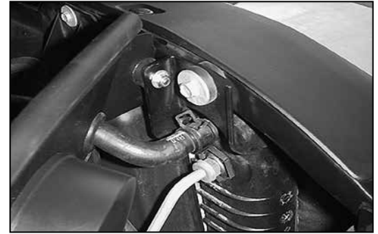
22. Secure the rubber mounted stud to the radiator mounting bracket.
