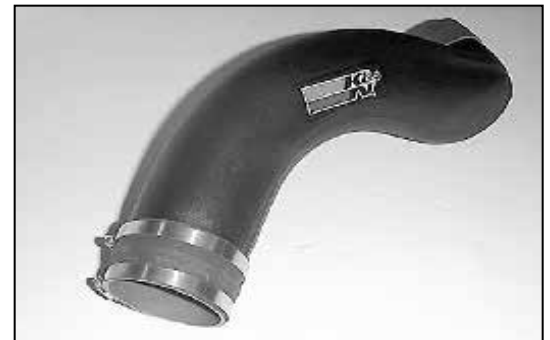
24. Install the 3.75"ID silicone hose (08631) onto the intake tube. NOTE: Do not tighten the hose clamps at this time.
