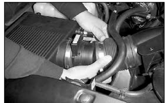
6. Detach the intake hose from the mass air sensor.
