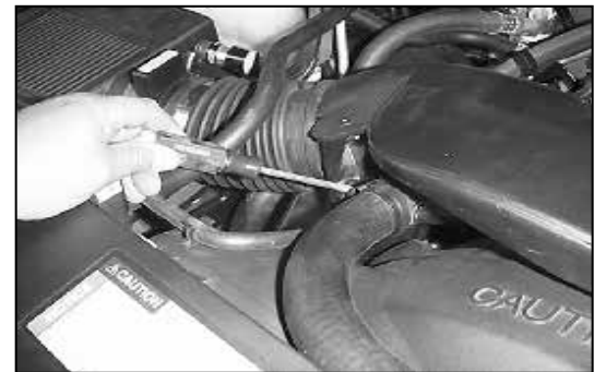
5. Using a flat blade screwdriver, pry the radiator hose retaining clip from the intake tube.
