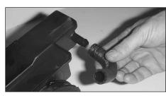
27. Detach the O.E. crankcase vent hose from the resonator
