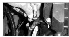
17. Install the 3/8"ID grommet onto the airbox mounting stud.
