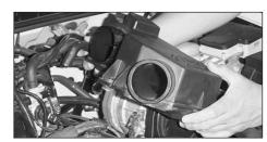
15. Detach the resonator from the throttle body and remove it.
