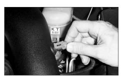
37. Reconnect the air temperature sensor electrical connection.
