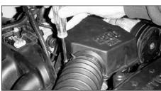
$5.\ \mbox{Loosen}$  the hose clamp on the intake hose at the resonator.
