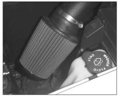
34. Install the filtercharger element and tighten hose clamp.
