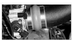
31. Attach the hump hose to the throttle body and tighten hose clamp.
