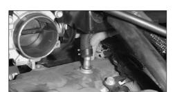
14. Detach the crankcase vent hose from the valve cover.
