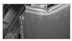
20. Secure the heat shield to the radiator core support using the clips removed in step 18.
