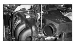
12. Loosen and remove the bolt that retains the resonator to it's mounting bracket.
