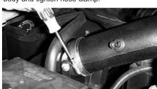
32. Secure the saddle bracket to the intake tube using the hose clamp provided.
