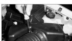
4. Loosen the hose clamp on the intake hose at the airbox.
