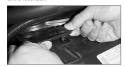
6. Pry up on the two push clips that retain the intake tube to the radiator shroud.
