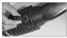
24. Remove the air temperature sensor from the stock intake hose.
