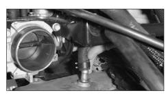
29. Attach the vent hose assembly to the vent fitting on the valve cover.
