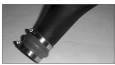
26. Attach the hump hose onto the K&N intake tube and tighten hose clamp.
