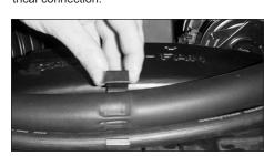
3. Detach the clip that retains the a/c lines to the radiator shroud.
