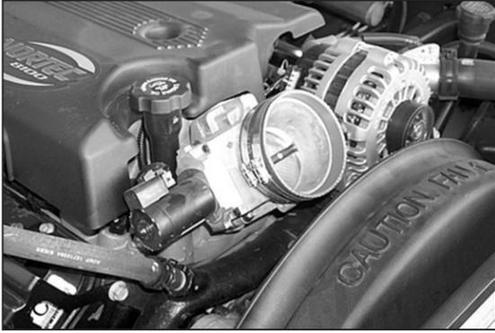
11. Install the silicone hose and hose clamps onto the throttle body as shown.
