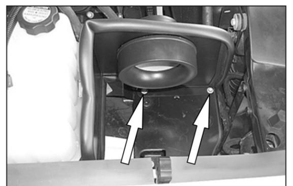
9. Using the two bolts removed in step 8, install the heat shield assembly as shown.
