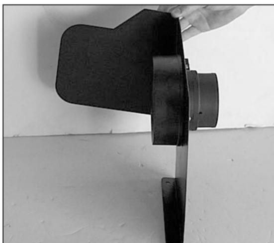
6. Using the provided hardware, assemble the mass air sensor, gaskets, heat shield and mass air sensor as shown.
