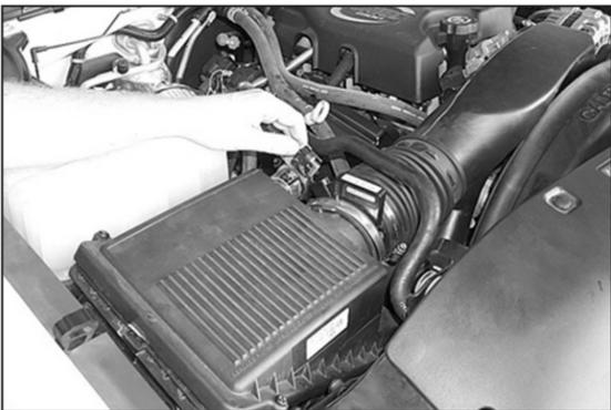
2. Disconnect the mass air electrical connection.
