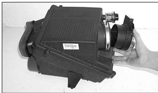
5. Loosen the hose clamp and remove the mass air sensor as shown.
