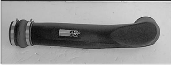
10. Install the silicone hump hose and hose clamps onto the K&N® intake tube as shown.
