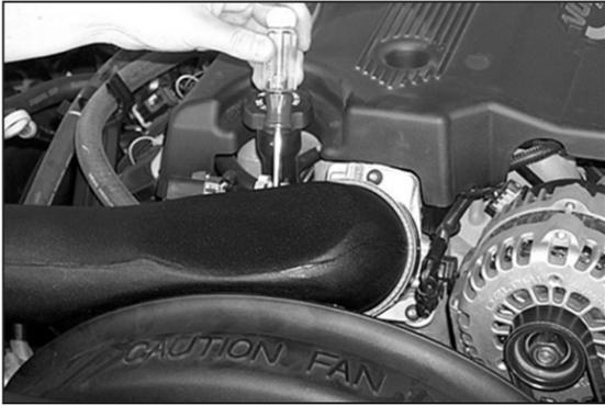
12. Slide the hump hose onto the mass air sensor then secure the other end to the throttle body as shown.
