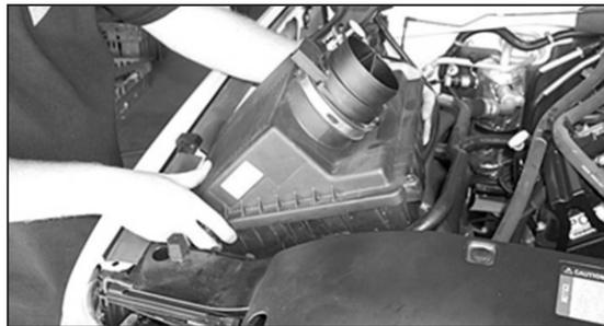
4. Pull firmly upwards to release the air cleaner assembly from the factory grommets, then remove the factory air cleaner assembly as shown.
