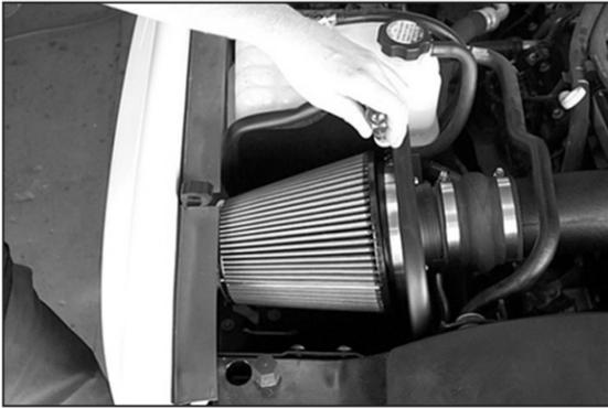
13. Install the K&N® Air Filter onto the mass air adapter, then tighten the hose clamp as shown.
