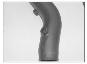
18a. On vehicles not equipped with a fuel pressure regulator vent hose, install the provided npt plug into the K&N<sup>®</sup> intake tube as shown.
