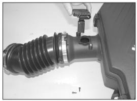
15. Remove the mass air sensor from the stock air box as shown.
