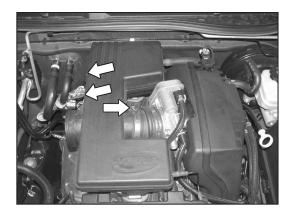
7. Loosen the two bolts that retain the intake resonator to the engine, then loosen the hose clamp at the throttle body.
