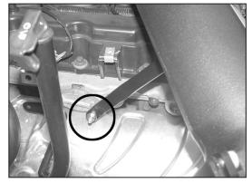
21. Install the tube mounting bracket onto the 6mm threaded stud protruding from the engine; secure with the provided washer and nut.
