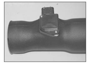
17. Install the mass air sensor assembly into the  $K\&N^{\circ}$  intake tube using the provided spacers and the provided button head allen bolts.
