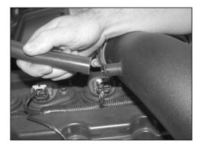
23. Install the provided crank case vent hose onto the valve cover, then onto the K&N $^{\mbox{\tiny (B)}}$  intake tube as shown.
