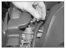
6. On vehicles equipped with a fuel pressure regulator vent hose, disconnect the fuel pressure regulator vacuum hose from the fuel pressure regulator as shown.
