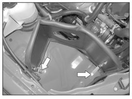
14. Install the heat shield into the vehicle using the provided hardware and the factory air box retaining nut.
