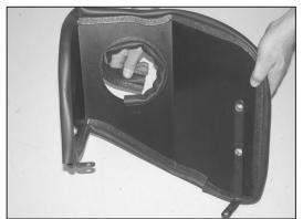
12. Install the edge trim onto the inner hole of the heat shield as shown. Trim if needed.
