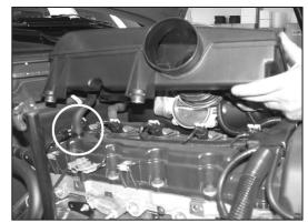
2. Depress the locking clip on the mass air sensor electrical connection and unclip the mass air sensor electrical connection.
