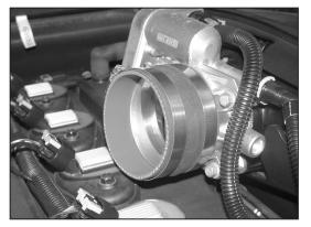
9. Install the silicone hose (08690) onto the throttle body and secure with the provided hose clamp as shown.
