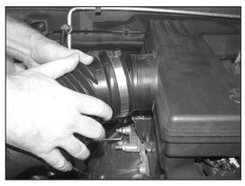
3. Loosen the hose clamp that retains the stock intake tube to the resonator, then remove the tube from the resonator as shown.
