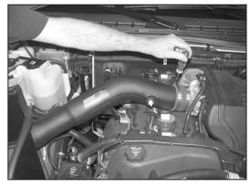
20. Install the K&N<sup>®</sup> intake tube into the silicone hose attached to the throttle body. Guide the intake tube through the heat shield and secure the hose clamps.
