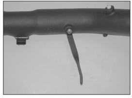
19. Install the mounting bracket onto the K&N<sup>®</sup> intake tube with the provided hardware as shown. **NOTE: Do not completely tighten at this time.**
