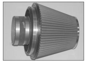
25. Install the silicone hose (08630) onto the air filter assembly as shown.
