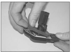
16. Apply provided gasket to mass air sensor as shown.
