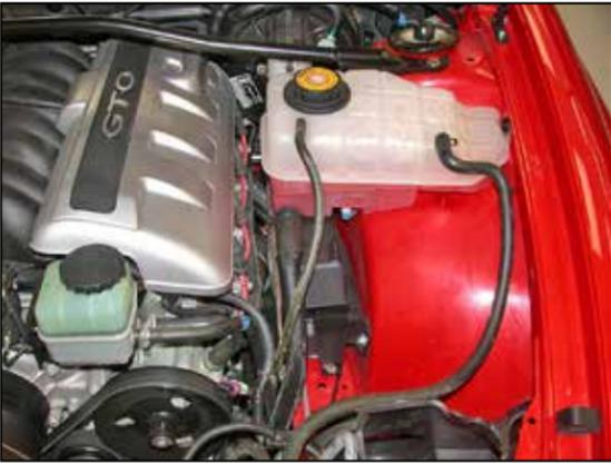
9. Reinstall the coolant reservoir onto the mounting studs as shown.
