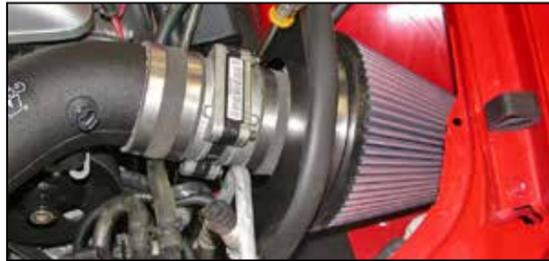
29. Install the air filter assembly onto the K&N® intake tube and secure with the provided hose clamp.
