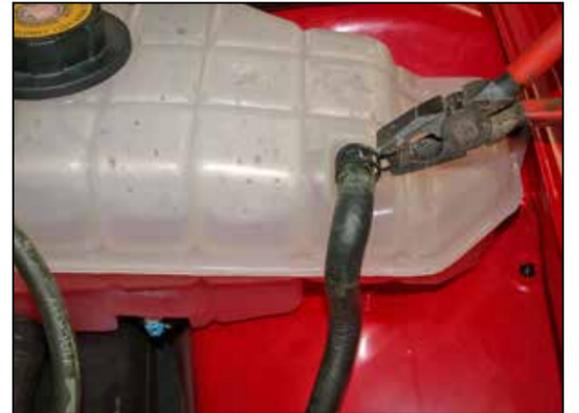
21. Using a pair of pliers, loosen the spring clamp on the coolant reservoir hose. rotate the coolant hose 90 degrees down as shown. Then resecure with the stock clamp.
