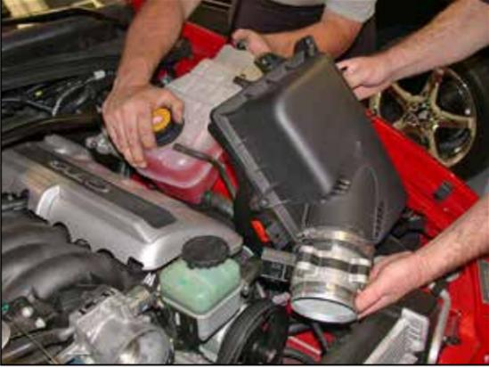
8. Have an assistant hold the coolant reservoir up, lift up on the air box assembly to release it from the retaining studs. Then remove the air box from the vehicle.
