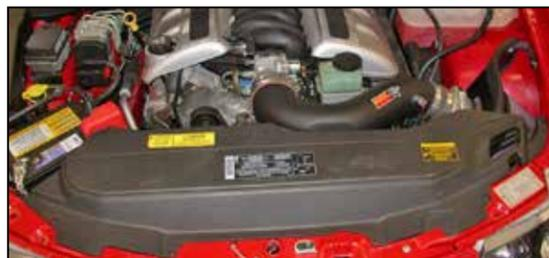
32. Reinstall the radiator cover removed in step #3.
