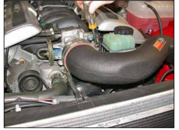
17. Install the K&N® intake tube onto the throttle body as shown and secure with the provided hose clamp, using the 8mm bolt provided. Secure the K&N® intake tube onto the mounting bracket installed in step #12.
