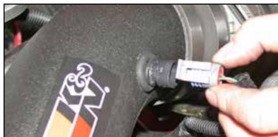
31. Reconnect the temperature sensor electrical connection.
