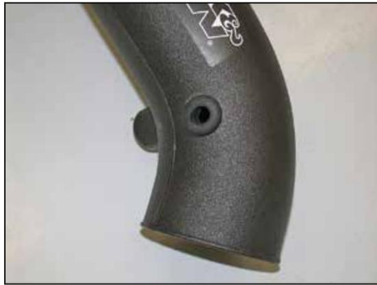
15. Install the provided rubber grommet into the K&N® intake tube as shown.
