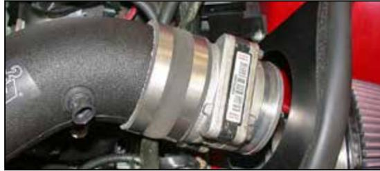
28. Install the mass air sensor assembly onto the K&N® intake tube and secure with the provided hose clamp.
