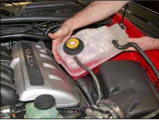
7. Pull the coolant reservoir up and away from the inner fender to release it from the retaining studs.
