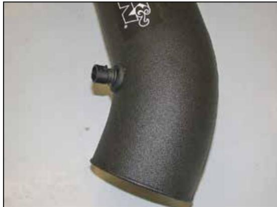
16. Install the air temperature sensor from step #14 into the grommet in the K&N® intake tube as shown.
