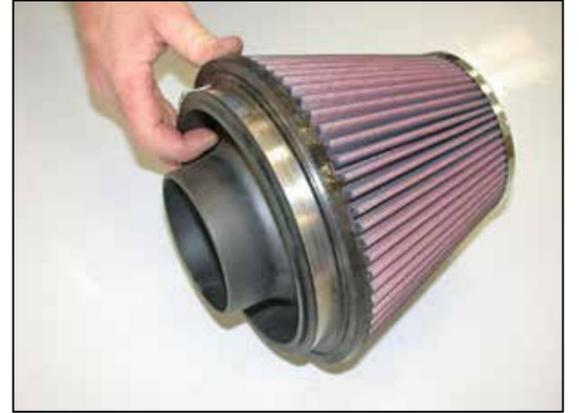
19. Install the radiused filter adapter into the K&N® air filter as shown. Secure with the provided hose clamp.
