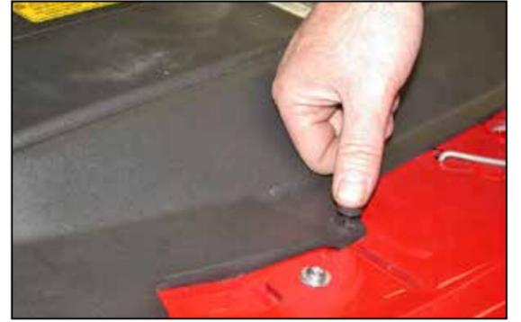
33. Reinstall the five radiator cover retaining clips removed in step #2.
