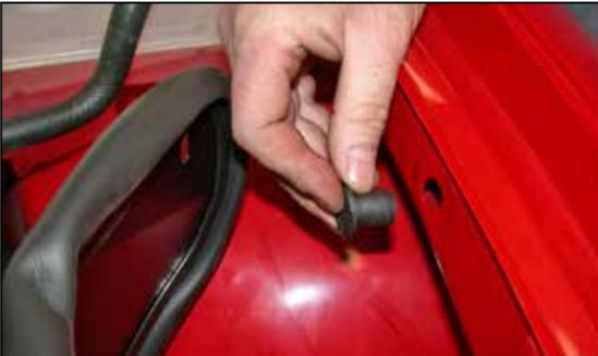
24. Install the threaded insert into inner fender as shown.
