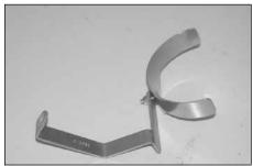
6. Install the saddle bracket onto the K&N® intake tube brackets as shown.
