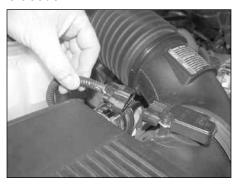
2. Depress the locking tab on the mass air sensor electrical connector, and then disconnect the electrical connection.
