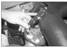
22. Reconnect the mass air sensor electrical connection as shown.
