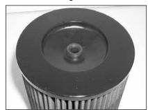
19. Install grommet onto filter as shown.
