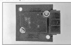
15a. Install the mass air sensor into the K&N® mass air sensor adapter and secure with the provided hardware.
