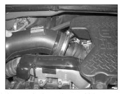
3. Loosen the hose clamp, which secures the intake tube to the intake manifold, and then disconnect the intake tube from the intake manifold.
