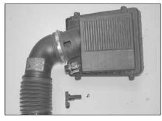
13. Using the "TORX" T20 wrench provided, loosen and remove the two-torx screw that retain the mass air sensor, and then remove the sensor.
