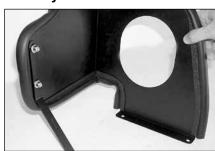
10. Install bracket onto heat shield as shown. Do not tighten completely.
