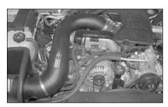
16. Secure the K&N<sup>®</sup> intake tube to the intake manifold with the provided hose clamp.
