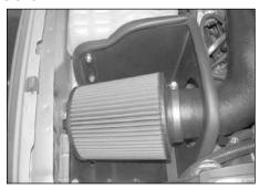
21. Install the K&N® air filter onto the intake tube as shown and tighten completely.
