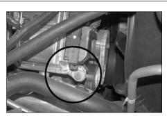
7. Remove the lower front engine processor mounting bolt shown.
