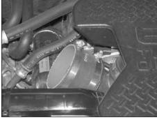
5. Install the silicone hose (08456) onto the intake manifold and secure with the provided hose clamps.
