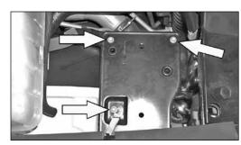
11. Remove the three bolts from the stock airbox mounting tray.
