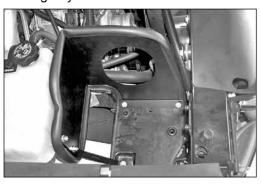
12. Mount the heat shield onto the airbox mounting tray and secure with the three bolts removed in step 10.
