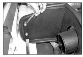
18. Adjust heat shield and bracket for necessary clearance, then tighten all hardware completely.
