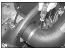
17. Install saddle bracket onto intake tube with hose clamp provided. Adjust for best fit and tighten all hardware.
