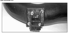
15b. Install the mass air sensor assembly into the K&N® intake tube and secure with the provided hardware.
