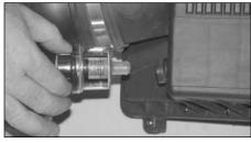
14. Remove the restriction gauge and grommet from the stock air box as shown.
