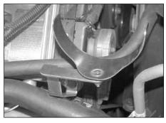
8. Using the factory bolt removed in step #7, install the tube-mounting bracket to the engine processor.
