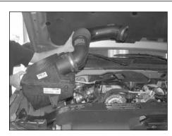
4. Lift up on the air box assembly to release from the mounting grommets, and then remove the air box and intake tube assembly from the vehicle.
