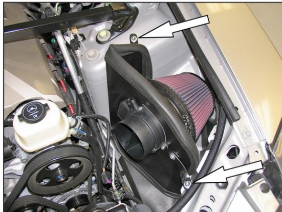
15. Install the heat shield and air filter assembly into the vehicle and secure with the provided hardware as shown.
