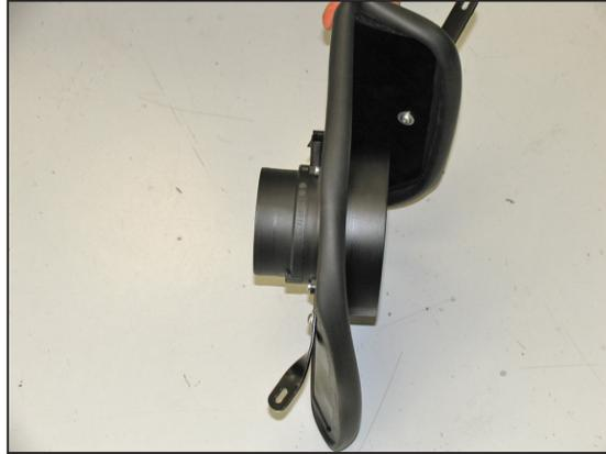
13. Install the mass air sensor onto the heat shield using the gaskets and filter adapter as shown.
