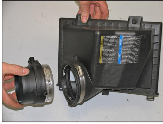
12. Loosen the hose clamp which secures the mass air sensor to the air box and then remove the mass air sensor from the air box as shown.
