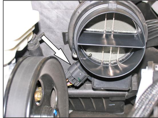
5. Disconnect the mass air sensor electrical connection shown.
