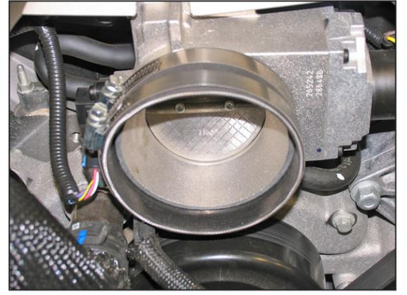
17. Install the silicone hose (08755) onto the throttle body and secure with the provided hose clamps.
