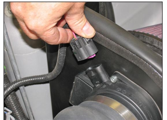
21. Reconnect the mass air sensor electrical connection as shown.
