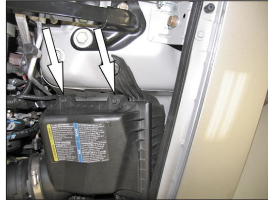
6. Loosen the two screws, which secure the air box lid to the air box base.
