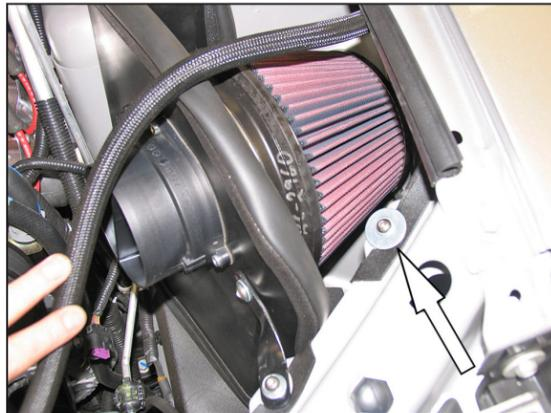
16. Install the provided button head allen and fender washer onto the core support to retain the inner splash shield as shown.
