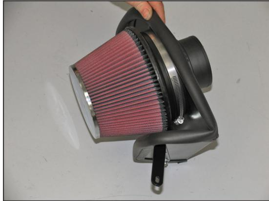
14. Install the K&N® air filter onto the heat shield assembly and secure with the provided hose clamp as shown.
