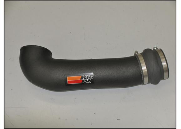
18. Install the silicone hump hose onto the K&N® intake tube as shown and secure with the provided hose clamp.
