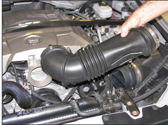
4. Loosen the two hose clamps which secure the intake tube to the throttle body and mass air sensor, then remove the intake tube as shown.
