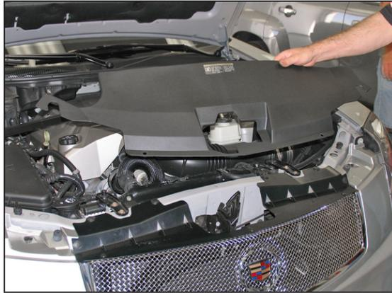
3. Dislodge the cover from the hold on clamps on the under side of the cover and then remove the cover as shown.
