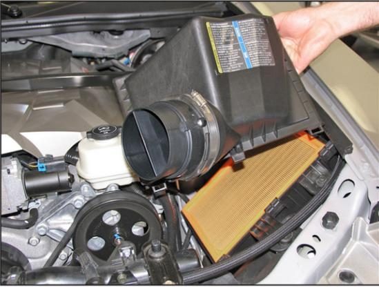
7. Lift and remove the air box lid and mass air sensor from the lower air box as shown.
