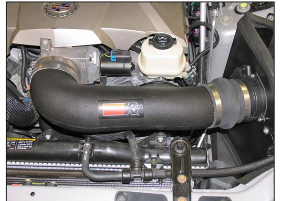
19. Install the K&N® intake tube onto the throttle body and mass air sensor as shown and secure with the provided hose clamp.
