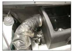
15. Install the fresh air supply hose onto the K&N<sup>®</sup> airbox and secure with the factory hose clamp.
