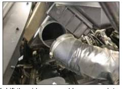
4. Lift the airbox assembly up enough to gain access to the fresh air supply hose clamp, then loosen the clamp and disconnect the fresh air supply hose from the airbox assembly.
