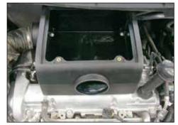
14. Install the K&N<sup>®</sup> airbox onto the engine. Using the supplied hardware, secure the airbox to the rear mounting bracket first and then to the coupling nuts installed in step #13.
