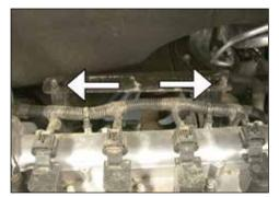
11. Remove the two stock airbox mounting anchors shown from the mounting bracket.
