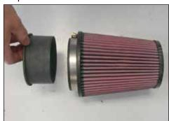
17. Install the filter adapter into the  $K\&N^{\ensuremath{\$}}air$  filter as shown.
