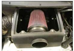
18. Place the filter assembly into the K&N<sup>®</sup> airbox as shown.
