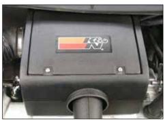
21. Install the K&N $^{\circ}$  airbox lid and secure with the provided hardware as shown.
