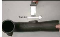
8. Install the mass air sensor into the intake tube as shown.
