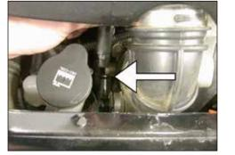
2. Loosen the hose clamp, which secures the crankcase vent hose to the stock intake tube, and
