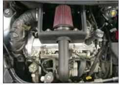
19. Install the K&N<sup>®</sup> intake tube through the opening in the airbox and into the filter assembly. Then install the intake tube into the silicone hose at the throttle body and secure the filter and tube with the provided hose clamps.
