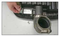
7. Remove the two screws securing the mass air sensor to the stock intake tube and then remove the sensor as shown.
