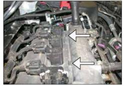
12. Install the two supplied 6mm studs into the valve cover as shown.
