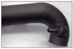
10. Install the supplied crankcase vent fitting into the intake tube as shown.
