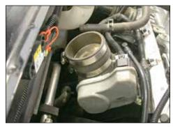
16. Install the silicone hose (08756) onto the throttle body and secure with the provided hose clamp.
