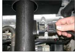
22. Reconnect the vehicles mass air sensor electrical connection.
