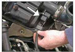
5. Flip the airbox assembly up towards the driver's side of the vehicle to gain access to the mass air
