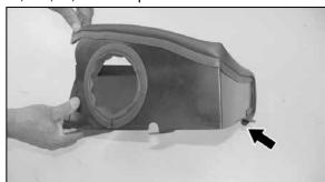
14. Starting at the rear-mounting tab, install the 32" long edge trim onto the heat shield as shown.
