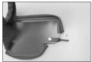
18. Install the mounting bracket onto the heat shield with the provided hardware as shown.
