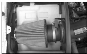
29. Install the K&N $^{\circledR}$  Air Filter onto the mass air sensor and secure with the provided hose clamp as shown.
