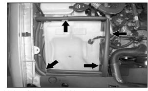
21. Install the heat shield onto the washer reservoir and secure the heat shield and mounting bracket with the provided hardware.
