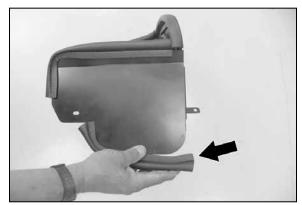
16. Install one of the 10" pieces onto the bottom of the front wall as shown.
