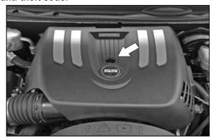
2. Remove the wing nut, which retains the engine cover and then remove the engine cover.
