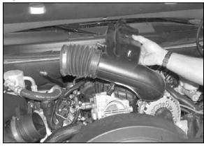
5. Disconnect the crankcase vent hose from the valve cover and then remove the stock intake tube as shown.
