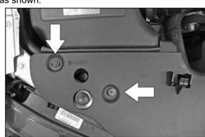
6. Remove the core support cover bolt and retaining clip shown.
