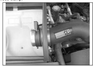
27. Install the mass air sensor assembly onto the intake tube and secure with the hose clamp provided.
