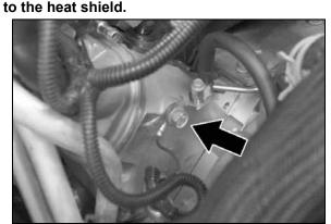
19. Remove the bolt, which secures the ground strap to the cylinder head shown.
