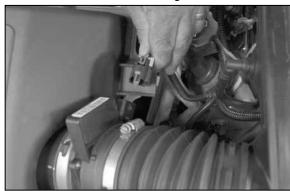
3. Depress the locking tab on the mass air sensor electrical connection and then separate the connector from the mass air sensor.
