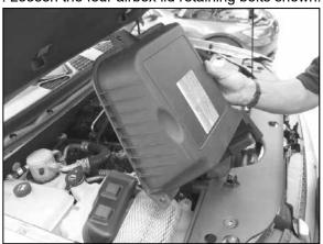
8. Lift up on the core support cover for clearance and then remove the airbox lid as shown.
