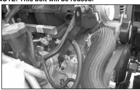
20. Using the bolt removed in step #19, secure the tube mounting bracket and ground strap to the cylinder head in the same location the bolt was removed from.
