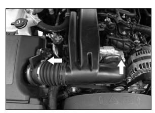
4. Loosen the two hose clamps, which secure the intake tube to the mass air sensor and throttle body.
