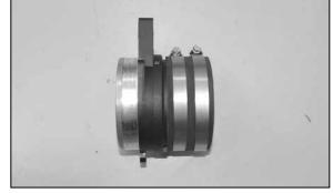
26. Install the silicone hose (08615) onto the mass air sensor as shown and secure with the provided hose clamp.
