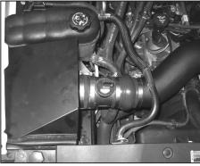
25. Install the air box lid and secure with the provided hardware.
