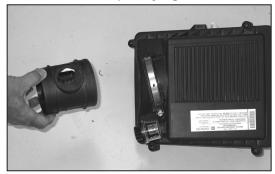
14. Loosen the hose clamp that secures the mass air sensor to the air box. Then remove the mass air sensor as shown.
