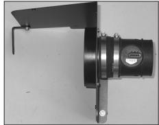
15. Install the mass air sensor onto the heat shield assembly and secure with the provided hose clamp.
