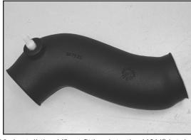
20. Install the  $\frac{1}{4}$ "npt fitting into the K&N® intake tube as shown.
