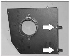
13. Install the two inserted nuts onto the heat shield as shown using the provided hardware.
