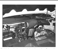
7. Unhook the stock intake tube from the mounting grommet and the upper radiator hose. Then remove the stock intake tube from the vehicle as shown.
