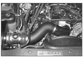
21. Install the K&N® intake tube into the throttle body and mass air sensor silicone hoses. Secure with the provided hose clamps.
