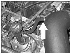
22. Install the supplied silicone hose onto the  $\frac{1}{4}$ "npt fitting installed into the K&N® intake tube and then attach the open end onto the crank case vent port on the valve cover.
