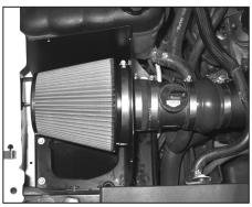
23. Install the  $K\&N^{\otimes}$  air filter onto the filter adapter and secure with provided hose clamp.
