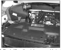
8. Firmly lift up the air box assembly to dislodge it from the mounting grommets. Then remove the air box assembly from the vehicle. NOTE: K&N Engineering, Inc., recommends
