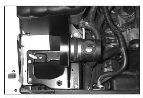
16. Install the heat shield assembly into the vehicle so that the inserted nuts fit into the air box mounting grommet holes. Then tighten the mounting bolts.
