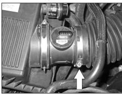
5. Loosen the hose clamp that secures the stock intake tube to the mass air sensor.
