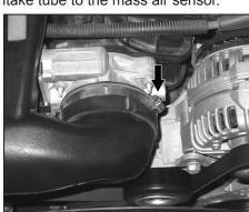
6. Loosen the hose clamp that secures the stock intake tube to the throttle body.
