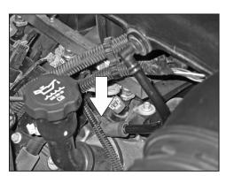
4. Disconnect the crank case vent hose from the valve cover vent port.
