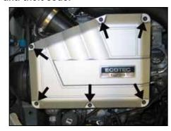
2. Remove the six TORX screws which secure the air box lid and then remove the air box lid from the vehicle.
