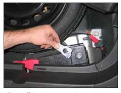
1. Turn off the ignition and then disconnect the negative battery cable. The battery is located in the trunk next to the spare tire.
