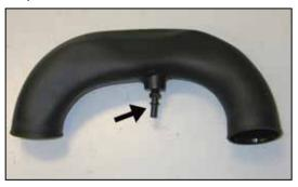
11. Install the provided crank case quick connect fitting into the K&N® intake tube as shown. **NOTE: Plastic NPT fittings are easy to cross**
