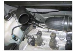
12. Install the K&N® intake tube into the silicone hose at the turbo inlet and secure with the provided hose clamp.
