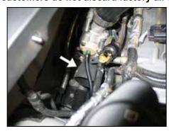
10. Install the provided silicone hose (08713) onto the turbo inlet and secure with the provided hose clamp.
