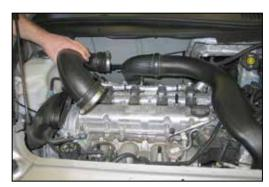
9. Loosen the hose clamp which secures the stock intake tube to the turbo inlet and then remove the intake tube from the vehicle.
