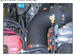
21. Install the K&N® intake tube into the silicone hose at the turbo inlet and then into the silicone hose at the mass air sensor. Adjust the tubes and mass air sensor housing for best fit and then secure with the provided hose clamps.
