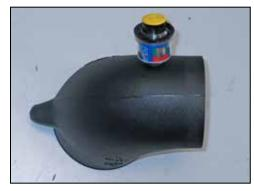
14. On vehicles equipped with a filter minder, remove the filter minder and grommet from the intake tube and install into the K&N intake tube as shown. On vehicles that are not equipped with a filter minder, drill the hole in the K&N intake tube out to 7/8"ID and then intall the provided plug into the tube.
