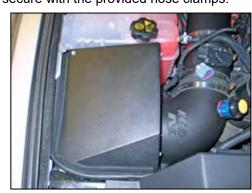
22. Install the heat shield lid onto the heat shield and secure with the provided hardware.
