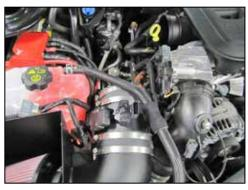
19. Install the mass air sensor assembly onto the K&N® intake tube as shown and secure with the provided hose clamp.
