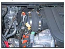
20. Install the provided hump hose (08617) onto the turbo inlet as shown and secure using the provided hose clamp.
