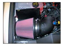
15. Install the K&N® intake tube into the heat shield and secure with the provided hardware. Then install the K&N® air filter onto the intake tube and secure with the provided hose clamp.
