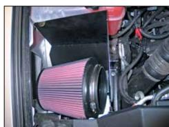
12. Carefully set the K&N<sup>®</sup> air filter into position on top of the air box tray.
