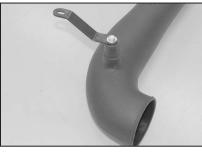
19. Install the tube mount bracket # 070065 onto the K&N $^{\mbox{\tiny B}}$  intake tube as shown.
