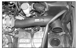
20. Set the K&N<sup>®</sup> intake tube in place through the heat shield but not onto the throttle body as shown.
