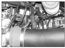
23. Install the provided silicone vent hose onto the  $K\&N^{\odot}$  intake tube and then install the crankcase vent tube into the silicone hose as shown.
