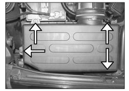
7. Loosen the four airbox lid retaining bolts shown.
