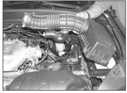
8. Remove the airbox lid and intake tube as shown.
