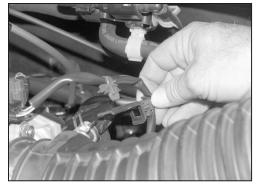
4. Unhook the wiring harness retaining clips as shown.
