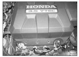
2. Turn the three-engine cover retaining screws 1/4 turn counter clockwise to unlock the cover from the engine.
