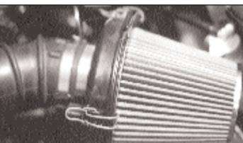
13b. On 1991-93 models, install the filtercharger assembly into the stock intake hose with the locating tab in the 12 o'clock position and secure with the hose clamp provided. Attach the saddle-bracket to the intake hose using the second hose clamp provided as shown above.
