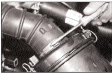
3. Loosen the hose clamp and disconnect the intake tube from the air cleaner assembly. **NOTE:** Remove the factory hose clamp as it will not be reused.
