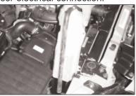
3. Slide the coolant reservoir tank up off it's retaining bracket and set it aside.
