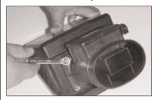
8. Loosen and remove the four nuts that secure the mass air sensor to the airbox top, then remove the mass air sensor.
