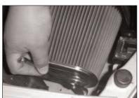
15. Secure the filter to the bracket with the provided hardware.
