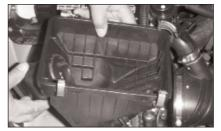
7. Remove the complete lower airbox inlet assembly as shown.
