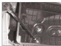
6. Loosen and remove the three bolts that secure the airbox base.
