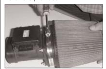
10. Attach the Filtercharger element onto the adapter and secure it with the provided hose clamp.
