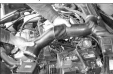
5. Remove the air intake tube as shown.
