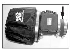
23. Install the silicone hose onto the mass air sensor with the provided hose clamps.
