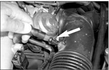
3. Disconnect the crank case vent as shown.
