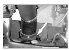
28. Install the mass air and filter assembly onto the intake tube. NOTE: when installing filter assembly it may be necessary to mount the filter assembly from under the vehicle.
