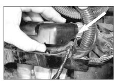
17. Trim the wire loom cover 45 degress to give the electrical lead clearance.
