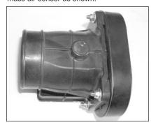
20. Install the K&N® filter adaptor onto the mass air sensor with the hardware provided.
