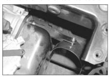
15b. Install saddle bracket assembly onto the transmission with the provided 10mm bolt. NOTE: make sure to install the provided spacer behind the new bracket.
