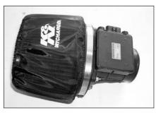
22. Install the provided dry charger onto the K&N® filter as shown.
