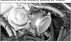
10. Install the silicone hose, (08756), onto the throttle body with the provided hose clamps as shown.
