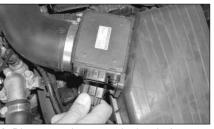
2. Disconnect the mass air electrical connection as shown.
