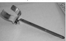
14. Vehicles that come equipped with manual transmissions assemble the large "L" bracket onto the saddle bracket as shown.
