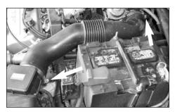
4. Loosen the hose clamp at the throttle body and air box assembly.
