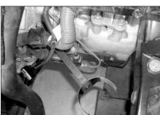
14b. Install the new saddle bracket assembly using the bolt that was removed in the previous step.
