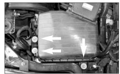
7. Loosen the three bolts that retain the air box onto
