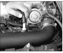
27. Reconnect the crank case vent onto the new K&N® intake tube as shown.
