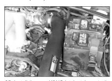
25. Install the new K&N® intake tube onto the throttle body. Do not tighten hose clamps completely at this time.
