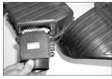
19. Remove the 4 nuts that retain the mass air sensor onto the factory air box then remove the mass air sensor as shown.
