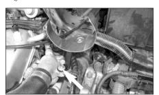
13. Secure the saddle bracket assembly onto the water neck with the provided bolt as shown.
