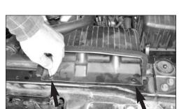
8. Remove the two push pins that retain the fresh air scoop onto the vehicle **NOTE**: To release the push pin press the center of pin to release.
