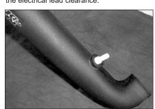
18. Install the vent fitting onto the new K&N® intake tube as shown.
