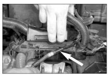
16. Release the 4 clips that hold the wire loom junction closed then lift up and remove the mass air electrical lead.
