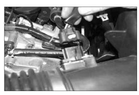
2. Disconnect the mass air sensor electrical connection and unhook the harness from the air box.
