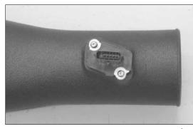
22. Install the mass air sensor into the K&N<sup>®</sup> intake tube and secure with the hardware provided.
