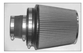
26. Install the silicone hose (08051) onto the air filter assembly as shown and secure with the hose clamp.
