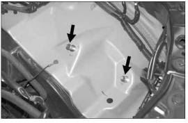
11. Remove the two air box mounting studs shown from the inner fender.
