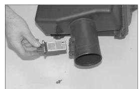
21. Remove the two screws, which secure the mass air sensor to the stock air box and then remove the mass air sensor from the air box.
