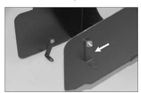
14. Install the "L" bracket (07805) onto the heat shield as shown with the provided hardware.
