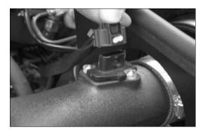
29. Reconnect the mass air sensor electrical connection.
