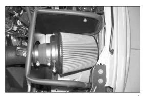
27. Install the air filter assembly onto the K&N® intake and secure with the provided hose clamp. NOTE: Drycharger® air filter wrap; part # RF-1014DK is available to purchase separately. To learn more about Drycharger® filter wraps or look up color availability please visit http://www.knfilters.com.
