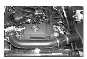
7. Loosen the two hose clamps shown which secure the stock intake tube to the air box and to the throttle body.
