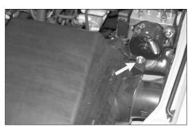
9. Remove the air box retaining bolt shown.
