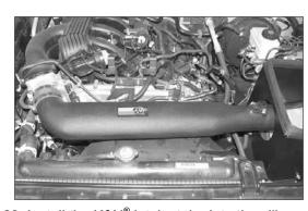
23. Install the K&N<sup>®</sup> intake tube into the silicone hose at the throttle body and align with the mounting bracket installed onto the heat shield. Secure the intake tube with the provided hardware.
