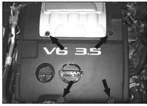
2. Remove the four bolts that retain the engine cover, then remove the engine cover from the engine.
