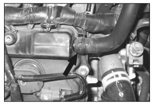
3. Release the spring clamp and disconnect the crank case vent hose.
