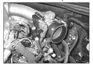
9. Install silicone hose (#08690) onto the throttle body and secure with the provided hose clamp.
