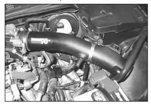
19. Install the K&N® intake tube assembly into the silicone hose at the throttle body and align with the saddle bracket installed in step #11. Secure the K&N® intake tube assembly with the provided hose clamps.
