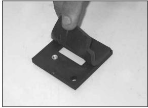
13. Install the provided gasket onto the  $K\&N^{\otimes}$  mass air sensor adapter.
