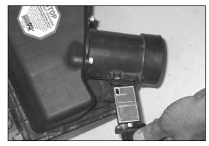
14. Remove the mass air sensor mounting screws. Then, remove the mass air sensor from the stock mass air sensor housing.
