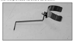
10a. On 2007 and later model vehicles, Secure the saddle clamp to the tube mounting bracket (070090) with the provided hardware as shown.
