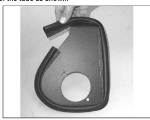
17. Install the provided edge trim onto the heat shield as shown.
