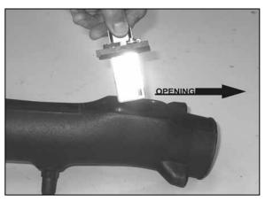
16. Install the mass air sensor assembly into the K&N® intake tube and secure with the provided hardware.
