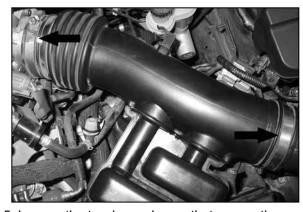
5. Loosen the two hose clamps that secure the stock intake tube to the throttle body and stock mass air sensor.
