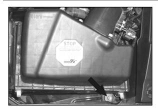
7. Remove the bolt that secures the air box to the inner fender.
