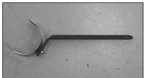
10. On 2004-2006 model vehicles, secure the saddle clamp to the tube mounting bracket (06489) with the provided hardware as shown.
