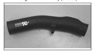
12. Install the  $1\!\!/\!_{\!4}$  '' NPT fitting into the K&N  $^{\!0}$  intake tube as shown.
