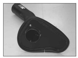
18. Secure the heat shield assembly to the K&N® intake tube with the provided hardware.
