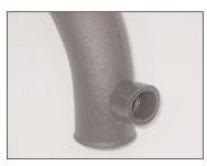
8c. Install the resonator grommet provided into the 1-3/8" hole drilled in step #8 as shown.
