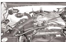
Disconnect the three hoses from the air box resonator and intake hose.
