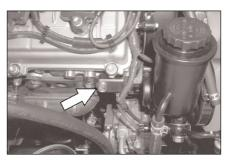
15a. On 2003 and later models, loosen and remove the bolt that secures the wire harness bracket located directly behind the power steering reservoir.
