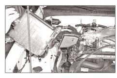
6. Remove the complete air intake system. NOTE: K&N Engineering, Inc., recommends that customers do not discard factory air intake.
