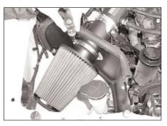
22. Install the K&N® air filter onto the K&N® intake tube and secure it with the provided hose clamp. NOTE: Drycharger® air filter wrap; part # RC-4700DK is available to purchase separately. To learn more about Drycharger® filter wraps or look up color availability please visit http://www.knfilters.com®.
