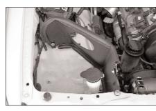
17. Install the heat shield and secure it to the new K&N® brackets with the hardware provided as shown. Do not tighten completely.
