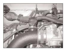
21a. On vehicles equipped with crank case vent resonator, connect the factory crank case vent hose onto the resonator as shown. NOTE: The crank case vent hose may need to be repositioned to enable it to reach the resonator.
