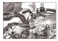
18. Install the silicone hose and hose clamps onto the throttle body as shown.
