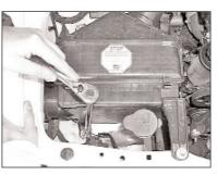
5. Loosen the three bolts that retain the air box assembly.
