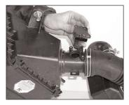
7. Loosen and remove the screws that secure the mass air sensor, then remove the mass air sensor.
