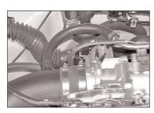
21. On 1999-00 models, attach the provided silicone hose onto the crankcase vent and connect it to the K&N® intake as shown.
