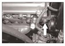
15c. On 2003 models, remove the bolt from power steering bracket as shown
