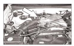
4. Loosen the hose clamps at the throttle body.
