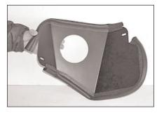
11. Install the two pieces of edge trim onto the heat shield as shown above.
