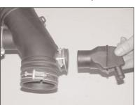
8a. On vehicles equipped with the crank case vent resonator chamber, loosen the hose clamp which secures the chamber to the intake tube and remove the chamber from the tube as shown.
