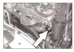
16a. On 2003 and later vehicles, install the saddle bracket assembly onto the motor using the bolt from step 15c. Do not tighten completely.
