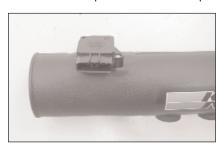
9. Install the mass air sensor into the K&N® intake tube using screws and spacers provided.
