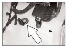
12. Install the "L" bracket onto the existing air box-mounting hole.
