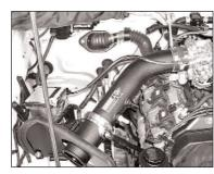
19. Install the K&N<sup>®</sup> intake tube onto the throttle body, and then tighten the hose clamps at the throttle body and saddle bracket.
