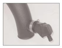
8d. Install the crank case vent resonator into the grommet installed in step #8c and secure with the provided hose clamp.
