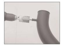
8b. On vehicles equipped with the crank case resonator chamber, using a 1-3/8" hole saw, drill out the 5/8" vent port as shown.
