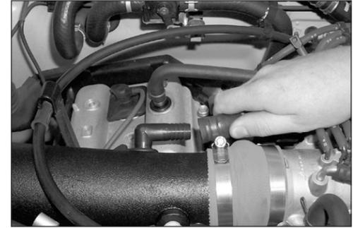
22. Vehicles equipped with the idle air vent line, reconnect vent line as shown.
