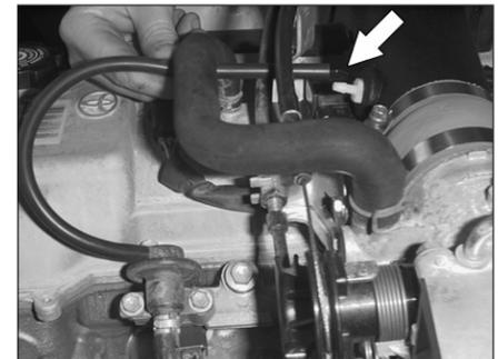
24. Install the provided silicone hose onto the fuel pressure regulator and connect the other end to the K&N® intake tube as shown.
