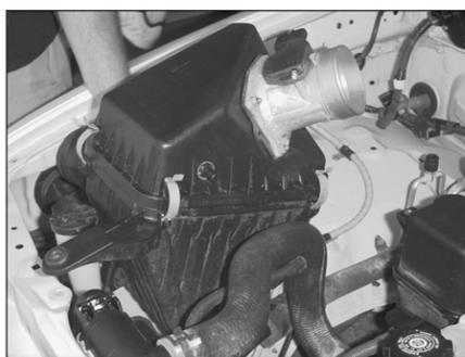
4. Loosen the three bolts that secure the air cleaner assembly, then remove the complete assembly as shown.
