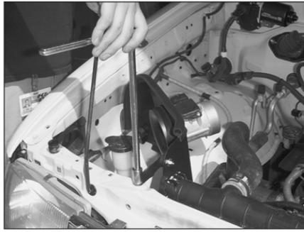
15. Install the heat shield assembly into the vehicle and secure it to the original air box mounting location as shown. Do not tighten completely. **NOTE: The fender washer and the rubber washer should be mounted between the fender and the "L" bracket.**
