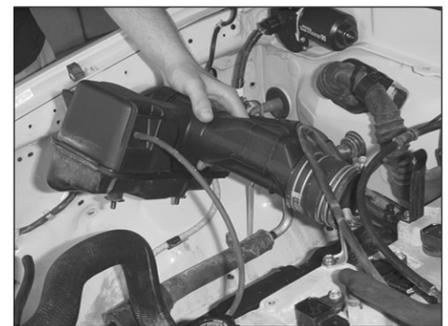
7. Loosen the hose clamp at the throttle body and remove the remaining section of the intake assembly.
