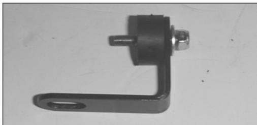
12. Assemble the rubber bumper stud onto the "L" bracket with the provided hardware as shown. **NOTE: Do not tighten completely.**
