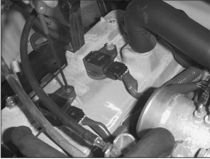
9. Replace the hex nut removed in step 8 with the provided button head screw and wave washer then secure the coil pack to the cam cover as shown.
