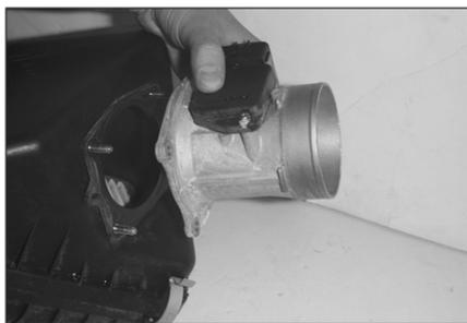
10. Loosen and remove the four hex nuts that secure the mass air sensor to the air cleaner assembly then remove the mass air sensor as shown.
