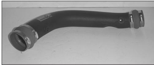
16. Secure the provided hump hoses onto the K&N® intake tube as shown using the provided hose clamp.
