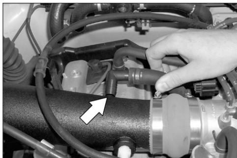
19. Vehicles equipped with an idle air vent line, install the 90 deg. fitting into vent line then mark the intake tube where the fitting lines up with tube. Vehicles that are not equipped with an idle air vent, continue on to step 23.
