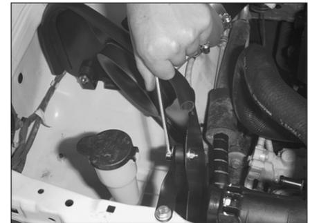
23. At this point, you can tighten the hardware located at the "L" and twist brackets as shown.
