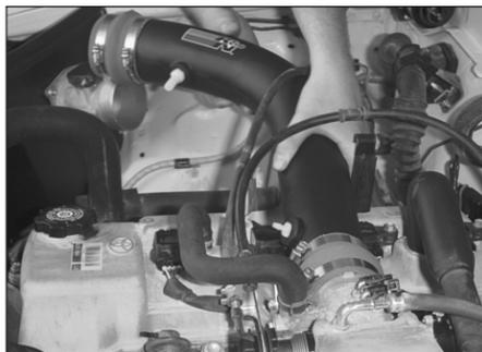
18. Install the intake tube onto the throttle body, then install onto the mass air sensor.
