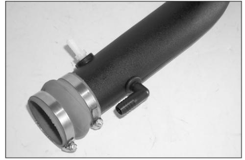
21. Install the 90 degree fitting into the intake tube as shown.
