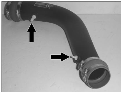
17. Install the two NPT fittings onto the K&N® intake tube as shown. **NOTE: Plastic NPT fittings are easy to cross thread. Install the vent fitting "hand" tight, then turn it two complete turns with a wrench.**
