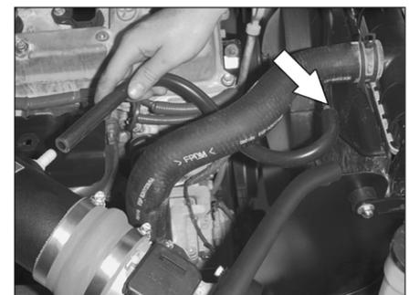
25. Install the provided silicone hose onto the EVAP canister vent and secure the other end onto the K&N® intake tube as shown.
