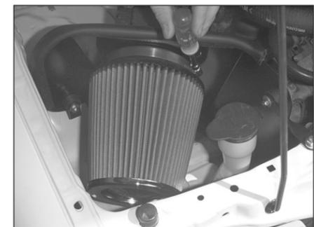
26. Install the K&N® air filter onto the mass air adapter and secure with the provided hose clamp as shown.
