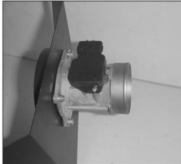
11. Assemble the mass air adapter, heat shield, gaskets and the mass air sensor using the hardware provided.
