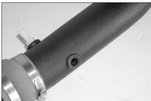
20. After marking the intake tube, remove from vehicle and drill a 7/8" hole into the intake tube then install the provided grommet as shown.
