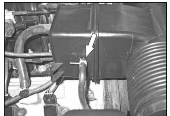
5. Release the spring clamp, then remove the P/S pressure switch vent hose from the intake tube.
