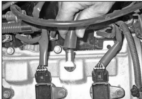
33. Install the remaining open end of the crank case vent hose onto the stock fitting on the valve cover.
