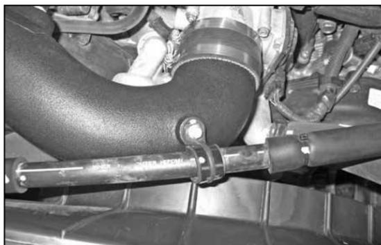
34. Fasten the A/C hose mounting clamp to the K&N® intake tube using the stock mounting bolt removed in step #4.
