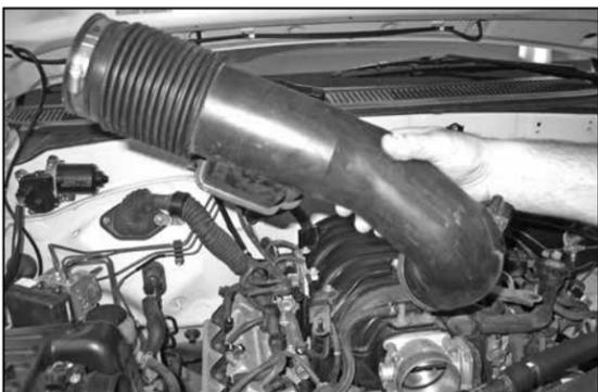
9. Remove the stock intake tube.
