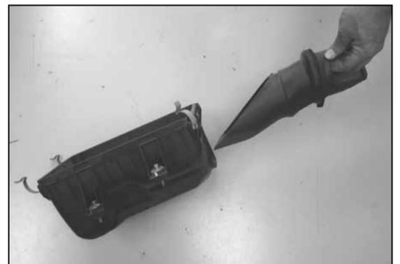
21. Remove the fresh air duct from the lower air box.
