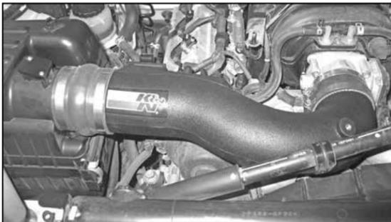
28. Install the K&N® intake tube into the silicone hoses previously installed onto the throttle body and air box.
