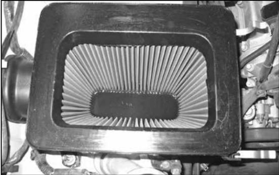
25. Install the K&N® air filter into the lower air box.
