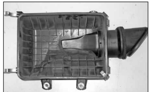
23. Re-install the fresh air duct into the lower air box and fasten with the provided hardware.
