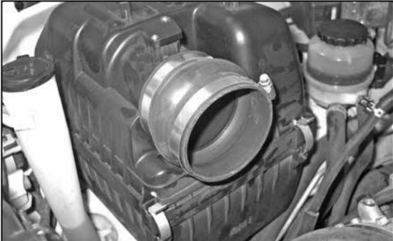
27. Install the provided silicone hump hose onto the air box and fasten with the provided hose clamp.
