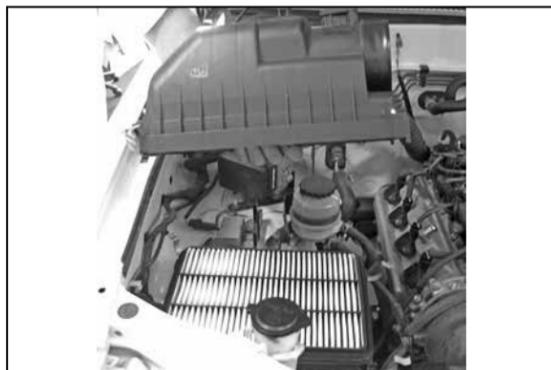
17. Release the four upper air box retaining clips, then remove the upper air box.
