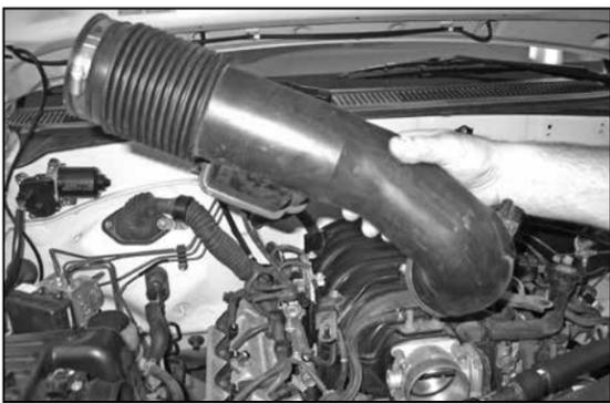
9. Remove the stock intake tube.
