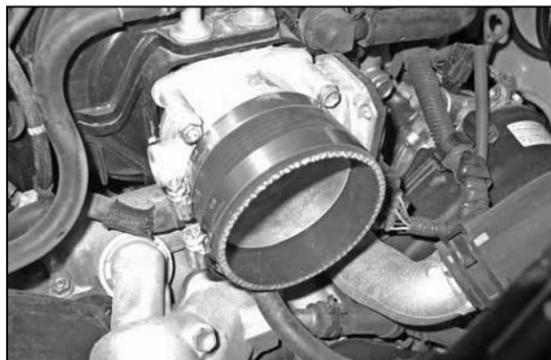
16. Install the provided silicone hose onto the throttle body and fasten using the provided hose clamp.
