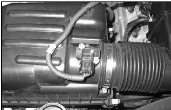
2. Disconnect the mass air sensor electrical connection, then release the mass air sensor wiring harness from the air box.
