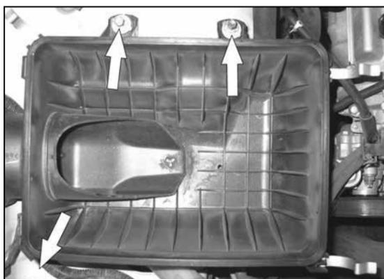
18. Remove the stock air filter, then remove the three bolts that secure the lower air box to the inner fender.
