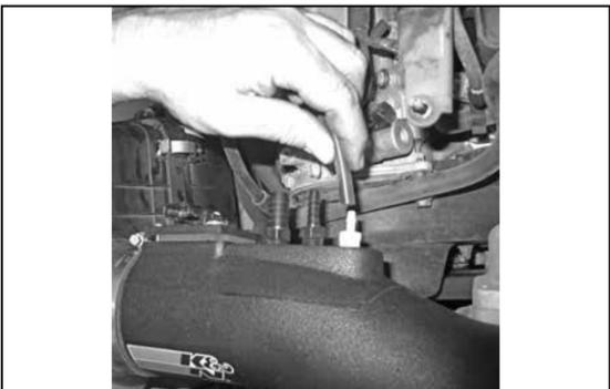
29. Install the provided 4mm silicone hose onto the npt vent fitting previously installed onto the K&N® intake tube.
