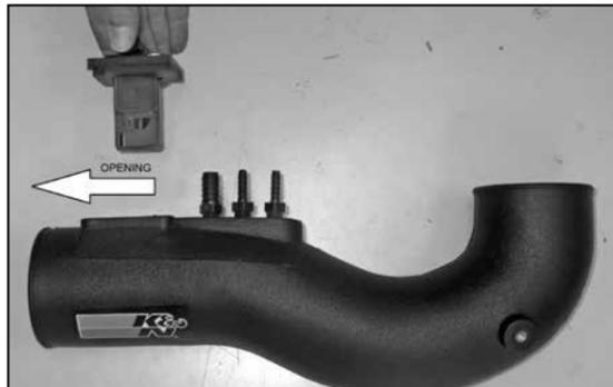
15. Install the mass air sensor assembly into the K&N® intake tube and fasten with the provided hardware.
