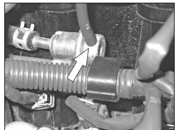
6. Disconnect the fuel pressure regulator vent line from the fuel pressure regulator.
