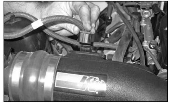
36. Re-connect the mass air sensor electrical connection. Secure the mass air sensor wiring harness to the intake tube with the tie wrap and bolt provided.
