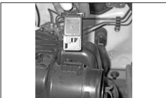
12. Remove the two screws that fasten the mass air sensor to the stock air box, then remove the mass air sensor.
