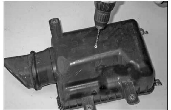
20. Drill out the center of the rivet that fastens the fresh air duct to the lower air box, then remove the rivet.
