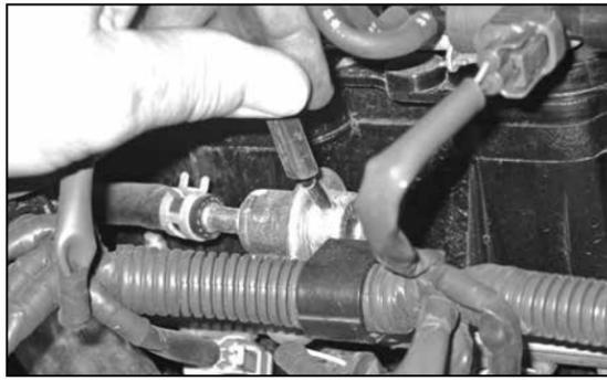
30. Connect the remaining open end of the 4mm silicone hose to the fuel pressure regulator vent port.
