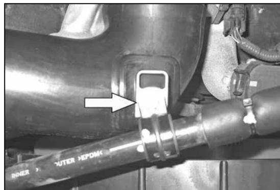
4. Remove the bolt that fastens the A/C mounting clamp.
