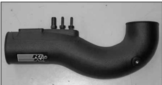
10. Install the three provided 1/4" npt fittings into the K&N® intake tube as shown.
