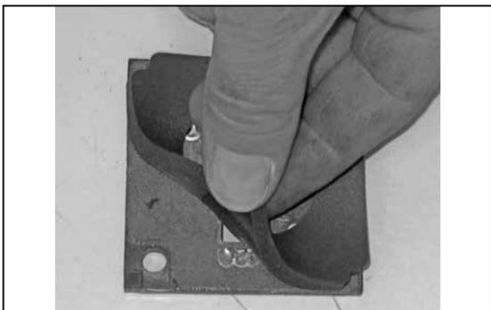
11. Install the provided gasket onto the K&N® mass air sensor adapter.
