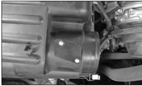
13. Install the provided mass air sensor block off plate onto the stock air box.
