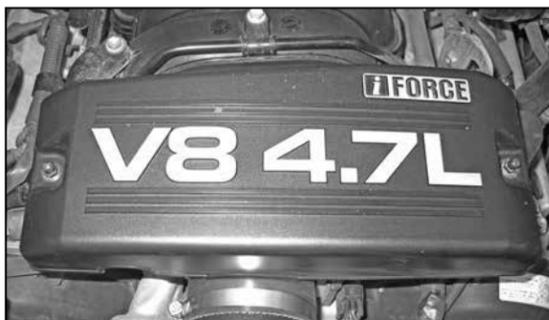
35. Install the stock throttle body cover and fasten using the stock nuts.
