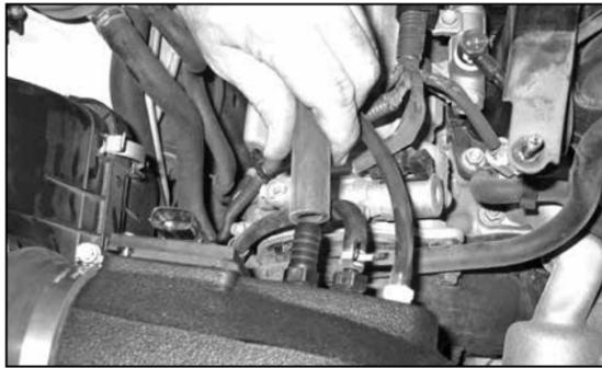
32. Install the provided crank case vent hose onto the npt fitting previously installed into the K&N® intake tube.
