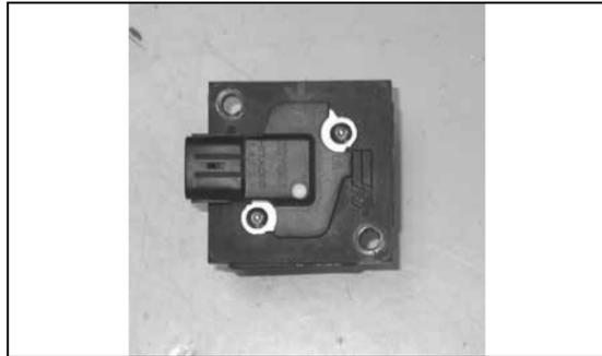
14. Install the mass air sensor into the K&N® mass air sensor adapter and fasten with the provided hardware.
