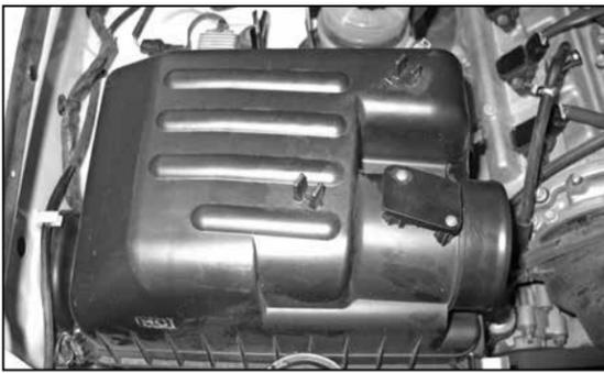
26. Install the upper air box and fasten with the stock retaining clips.
