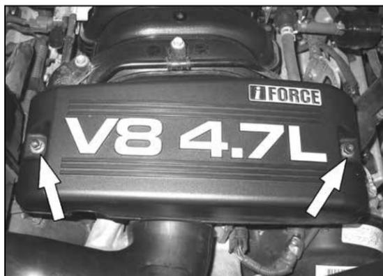
3. Remove the two nuts that fasten the throttle body cover, then remove the throttle body cover.
