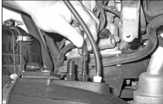
31. Connect the P/S pressure switch vent hose to the npt fitting previously installed into the K&N® intake tube, then fasten using the stock spring clamp.
