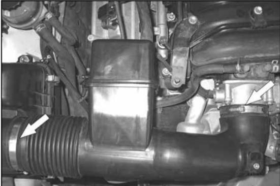
8. Loosen the hose clamps that fasten the stock intake tube to the throttle body and air box.
