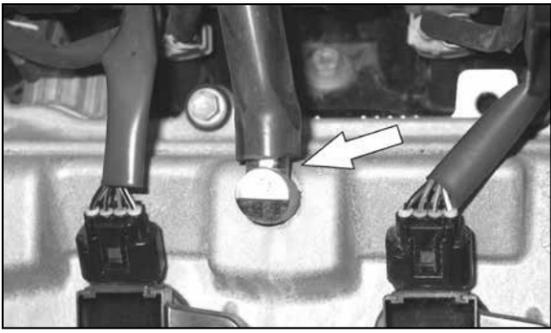
7. Disconnect the crank case vent hose from the valve cover.
