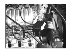
7. Disconnect the four rubber hoses from the engine as shown by the arrows. NOTE: Some '03 models may come equipped with only three vacuum lines.
