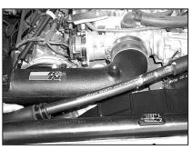
24. Install the K&N<sup>®</sup> intake tube onto the throttle body and secure with the provided hose clamp.
