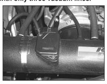
28. Attach the three provided, and one existing hose onto the  $K\&N^{\odot}$  intake tube as shown. NOTE: Some '03 models may come equipped with a total of three vacuum lines.
