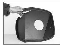
12. Apply the edge trim to the K&N<sup>®</sup> heat shield as shown above, trim if needed.
