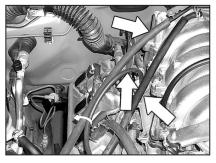
27. Install the three vent hoses onto the engine as shown above. (see arrows) NOTE: Some '03 models may come equipped with only three vacuum lines.
