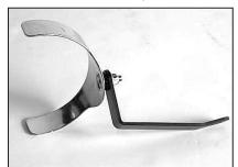
21. Assemble the saddle bracket assembly as shown above.
