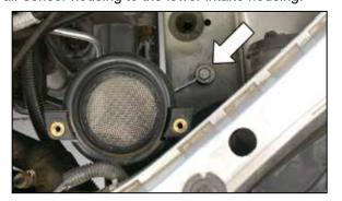
8. Remove the bolt, which secures the mass air sensor housing bracket to the inner fender.
