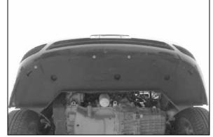
30a. On vehicle's that were equipped with the splash shield, reinstall with the bolts removed in step #10a.
