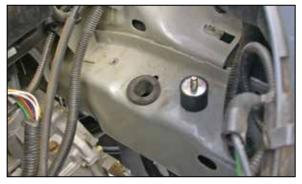
25. Install the rubber mounted stud into the threaded hole in the frame rail as shown.
