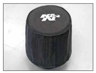
28. Install the provided Drycharger® onto the air filter as shown.
