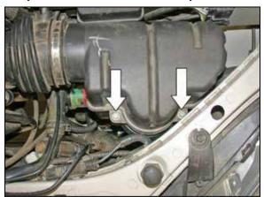
4. Loosen the two bolts, which secure the upper intake housing to the mass air sensor housing.
