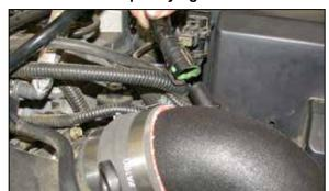
27. Reconnect the crank case vent hose to the fitting installed into the K&N® intake tube in step #18.
