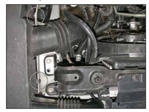
11. On vehicle's equipped with an air box cover, remove the two bolts which secure the cover to the frame rail, and the bolt which secures the intake snorkel to the radiator core support.
