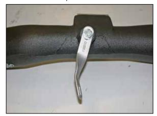
24. Install the provided bracket (010063) onto the K&N® intake tube with the provided hardware as shown.
