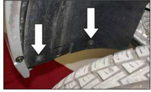
10. After jacking up the car and placing on suitable jack stands and chocking the rear wheels, remove the two bolts which secure the air box on equipped vehicle's or the one bolt on splash shield equipped vehicle's to the inner finder well.
