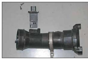
19. Remove the mass air sensor from the factory mass air sensor housing using the Torx wrench provided.
