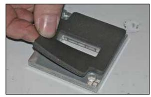
20. Apply the provided gasket onto the K&N® mass air adapter as shown.
