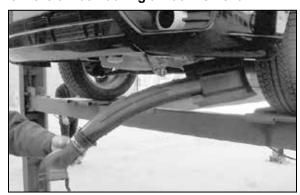
14a. On vehicle's equipped with the upper intake snorkel, pull down on the snorkel to dislodge it from the mount and then remove it from behind the fonder.
