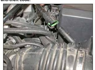
2. Depress the green locking tab on the crank case vent hose and then pull the vent hose to disconnect from the fitting as shown.
