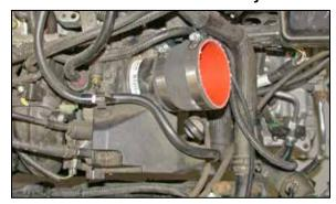
15. Install the silicone hose (08192) onto the throttle body and secure with the provided hose clamp.
