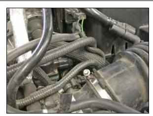
3. Loosen the hose clamp, which secures the factory intake tube to the throttle body.
