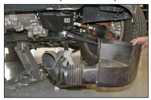
30. On vehicle's that were equipped with an air box cover, reinstall and secure with the bolts that were removed in step #11.
