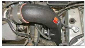
26. Install the K&N® intake tube assembly into the silicone hose at the throttle body and onto the rubber mounted stud, then secure with the provided hardware.
