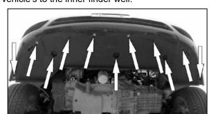
10a. On vehicle's equipped with the splash shield, remove the six bolts and five plastic screws which secure the splash shield to the bumper cover, then remove the splash shield from the vehicle.
