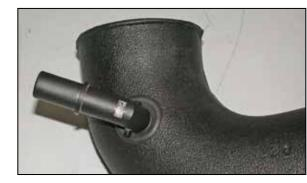
18. Install the crank case vent fitting removed in step #16 into the grommet installed into the K&N® intake tube in step #17 as shown.
