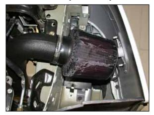
29. Install the air filter onto the K&N® intake tube and secure with the provide hose clamp.
