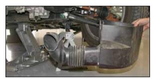
12. On vehicles equipped with an air box cover, lower the cover and remove it from the vehicle.
