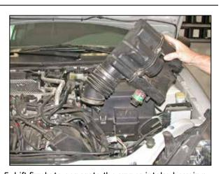
5. Lift firmly to separate the upper intake housing from the mass air sensor housing and then remove the upper intake housing from the vehicle.
