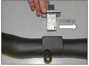
22. Install the mass air sensor assembly into the  $K\&N^{\scriptsize \$}$  intake tube.
