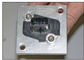
21. Using the factory mass air bolts, install the mass air sensor into the K&N<sup>®</sup> mass air adapter as shown.
