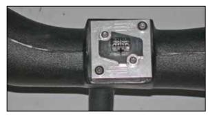
23. Secure the mass air sensor assembly into the K&N® intake with the provided hardware as shown.
