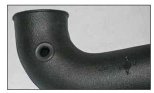
17. Install the provided grommet into the K&N® intake tube as shown.
