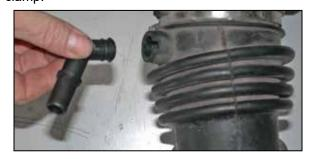
16. Remove the crank case vent fitting from the factory intake tube as shown.
