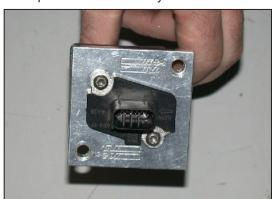
13. Using the factory mounting screws, install mass air sensor into the  $K\&N^{\otimes}$  adapter assembly as shown.
