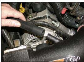
23. Install the provided crankcase vent hose onto the fitting at the valve cover then attach the other end to the port on the K&N® intake tube.
