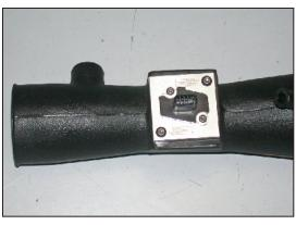
15. Secure the mass air assembly onto K&N® intake tube using the hardware provided as shown.
