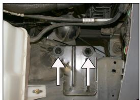
9. Remove the two-airbox mounting grommets from the mounting plate shown.
