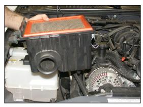
7. Pull firmly up on the lower airbox housing to dislodge from the mounting grommets and remove lower airbox from the vehicle.
