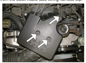
3. Remove the three- engine cover mounting bolts shown.
