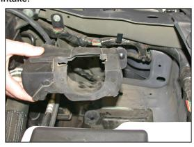
8. Pull firmly on the air duct to dislodge it from core support and remove from the vehicle.
