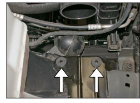
21. Install the two provided threaded inserts into the lower airbox mounting plate at shown.
