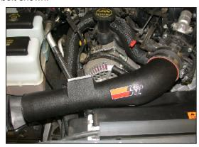
18. Install the K&N® intake tube into the silicone hose at the throttle body and secure the bracket in place on the alternator with the bolt removed in step #17.
