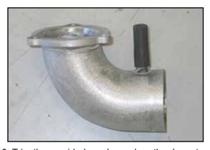
8. Trim the provided crankcase breather hose to a length of 1.5" and then install it onto the K&N $^{\circ}$  intake tube as shown.
