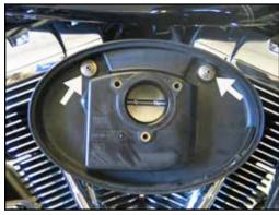
5. Remove the two breather / air filter base mounting bolts shown.
