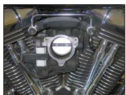
7. Install the supplied crankcase breather tube using the provided breather bolts and washers.
