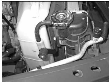
16. On 2008 & earlier vehicles install the "L" bracket (26607) onto the fan shroud with the provided 8mm bolt and washers.
