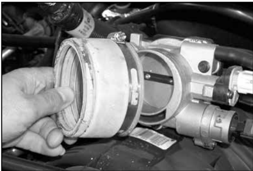
8. On 2002-2007 model year vehicles, loosen hose clamp that retains the rubber hose to the throttle body then remove as shown.
