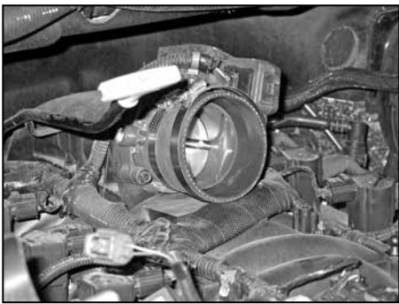
8a. Install the provided silicone hose (08051) onto the throttle body and secure with the provided hose clamp.
