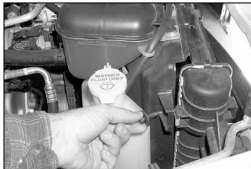
15. On 2008 & earlier vehicles, remove the 13mm bolt from the upper fan shroud as shown.
