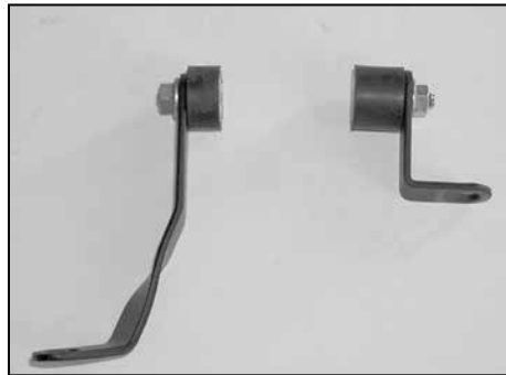
13. Install the rubber mounted studs into the provided brackets as shown
