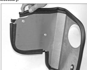
19. Install the long edge trim onto the heat shield assembly as shown.
