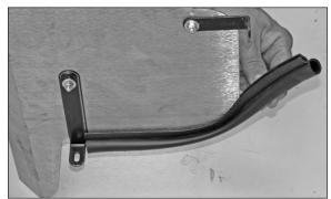
18. Install the short edge trim onto the heat shield assembly as shown.
