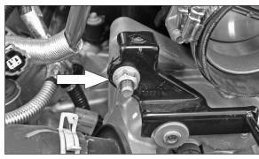
23. Remove the nut, which secures the intake plenum-mount shown.
