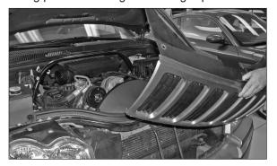
11. Remove the six grill retaining clips from the grill, then tilt the grill forward and lift to remove from the vehicle.
