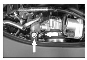
4. Remove the intake plenum-mounting bolt and loosen the intake plenum hose clamp at the throttle body.
