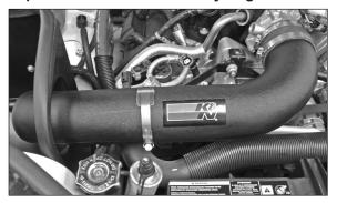
30. Install the intake tube into the silicone hose at the throttle body and onto the saddle clamp, then secure with the provided hose clamps.
