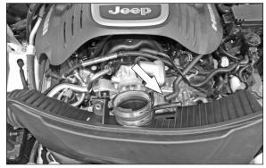
5. Pull the intake plenum off the throttle body and rotate forward, then disconnect the crank case vent hose from the tube attached to the intake plenum.
