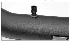
29. Install the air temperature sensor into the intake tube as shown.
