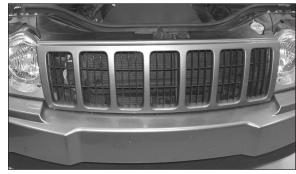
36. Reinstall the grill assembly with the factory retaining clips removed in step #5.
