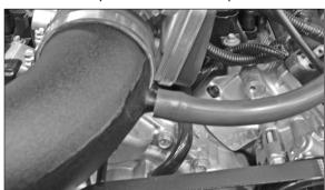
31. Install the provided crank case vent hose onto the valve cover and then onto the intake tube as shown.
