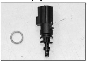
28. Remove the rubber sealing "O" ring from the air temperature sensor as shown.
