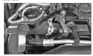
25. Install the tube mounting bracket assembly onto the plenum mount and secure with the factory nut removed in step #23.
