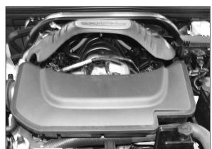
3. Remove the oil filler cap and then lift up the front of engine cover to gain access to the throttle body hose clamp intake plenum mounting bolt.
