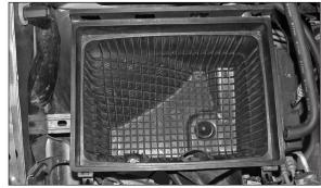
13. Remove the air box mounting bolt shown.
