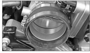
22. Install the silicone hose (08630) onto the throttle body and secure with the hose clamp provided.
