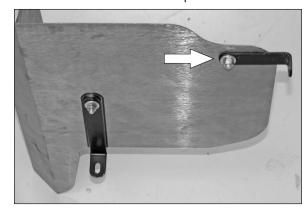
17. Install the small "L" bracket (07158) onto the heat shield as shown with the provided hardware.
