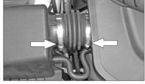
2. Loosen the hose clamp, which secures the stock intake tube to the intake plenum, and disconnect the crank case vent hose form the air box lid.
