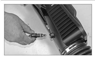
27. Rotate the air temperature sensor counter clockwise and remove the sensor from the stock intake plenum as shown.
