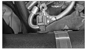
32. Reconnect the air temperature sensor electrical connection as shown.
