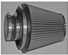
34. Install the silicone (08630) onto the air filter assembly and secure with the provided hose
