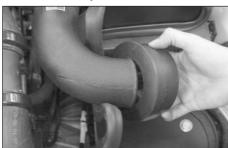
18. Install the air filter adaptor onto the intake tube as shown.
