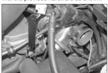
12. Install the provided silicone hose (08405) onto the turbo inlet as shown with the provided hose clamp.
