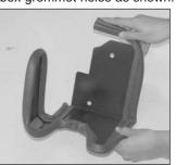
10. Install the edge trim onto the heat shield as shown. Trim if needed.
