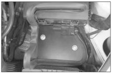
11. Install the heat shield onto the vehicle with the provided hardware as shown.
