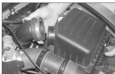
2. Loosen hose clamp at the air box, then remove intake tube from the air box as shown.
