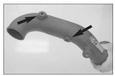
13. Install the two provided grommets onto the intake tube as shown.
