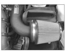
19. Install the air filter onto the intake tube as shown.
