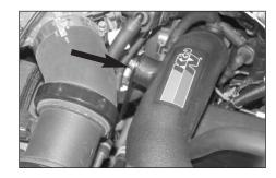
17. Connect the new intake tube onto the turbo inlet with the provided hose clamp. Then connect the intake tube to the bracket on the cylinder head as shown.
