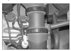
15. Connect the silicone hose with vent fitting on the valve cover as shown.
