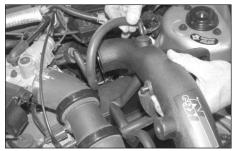
16. Reconnect the two vent fittings onto the new intake tube as shown.
