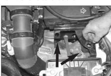
7. Remove the two air box grommets from the stock air box mounting tray.
