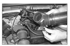
5. Disconnect the vacuum line from the intake tube as shown.
