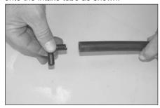
14. Install the 90 deg vent fitting onto the provided silicone hose as shown.
