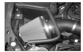
24. Install the K&N<sup>®</sup> air filter assembly on the intake tube and secure with the provided hose clamp as shown.
