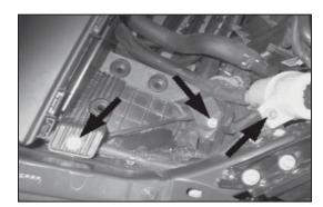
13.Remove the power steering reservoir mounting bolt and the two airbox bracket mounting bolts shown.
