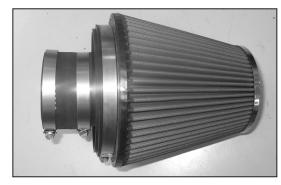
23. Install the silicone hose (08630) onto the air filter adapter and secure with the provided hose clamp.
