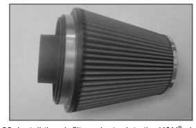
22. Install the air filter adapter into the K&N $^{\!0}$  air filter and secure with provided hose clamp.
