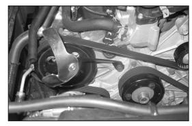
12. Install the tube mounting bracket assembly onto the engine and secure with the bolt removed in step #10.
