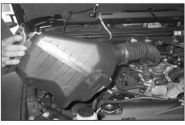
5. Lift up the airbox assembly to dislodge it from the mounting grommets and then remove the complete assembly from the vehicle.
