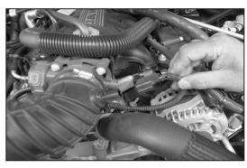
2. Release the locking tab on the air temperature sensor electrical connector and then disconnect the connection.
