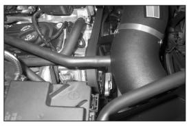
21. Connect the crankcase vent hose to the intake tube.
