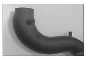
8. Install the air temperature sensor into the grommet installed into the intake tube during step #6.
