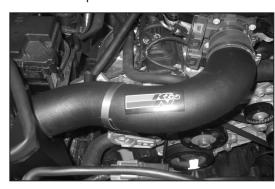
20. Insert the intake tube into the silicone hose at the throttle body and align with the mounting bracket installed in step #12 and then secure with the hose clamps provided.
