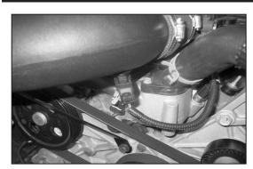
25. Reconnect the air temperature sensor electrical connection.
