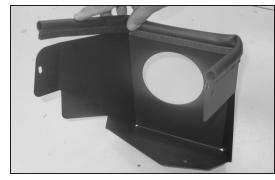
14. Install the supplied edge trim onto the heat shield as shown.
