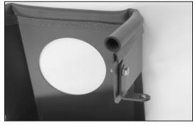
17. Install the supplied "L" bracket (070712) onto the heat shield as shown with the provided hardware. NOTE: The bracket should be installed on the outside of the heat shield with the "L" portion pointing towards the outside of the heat shield.
