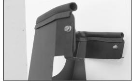
18. Install the supplied "L" bracket (07195) onto the heat shield as shown with the provided hardware.
