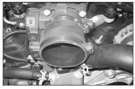
9. Install the supplied silicone hose onto the throttle body and secure with the supplied hose clamp.
