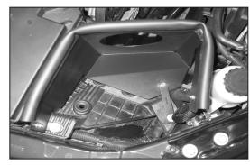
19. Install the heat shield assembly into the engine compartment and secure with the three bolts removed in step #12.
