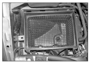
10. Remove the air box mounting bolt as shown.
