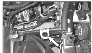
12. Remove the stock air box mounting grommet as shown.
