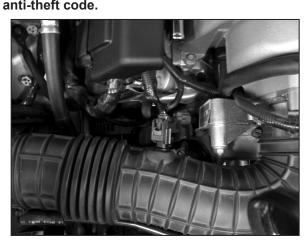
2. Release the red locking tab and disconnect the air temperature sensor electrical connection as shown.
