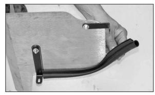
19. Install the short edge trim onto the heat shield assembly as shown.
