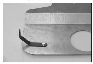
16. Install the provided "C" bracket (#07171) onto the heat shield with the provided hardware as shown.
