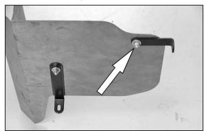
18. Install the small "L" bracket (#07158) onto the heat shield with the provided hardware as shown.
