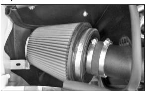
32. Install the K&N® air filter assembly onto the K&N® intake tube and secure with the provided hose clamp as shown.
