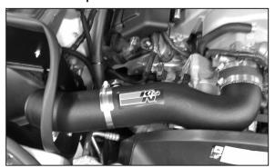
27. Install the K&N® intake tube into the silicone hose on the throttle body and align with the saddle clamp. Then, secure the intake tube with the provided hose clamps.
