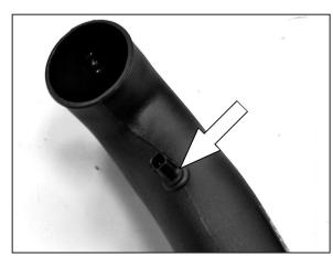
25. Install the air temperature sensor into the grommet installed into the K&N® intake tube in the previous step.
