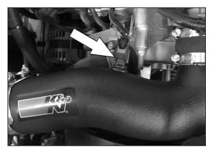
29. Re-connect the air temperature sensor electrical connection.
