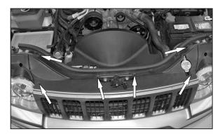
7. Using a small screw driver, release the center holding pins in the six grille retaining clips as shown.
