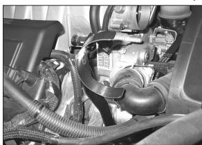
15. Install the tube mounting bracket assembly onto the upper alternator mount using the bolt removed in the previous step.
