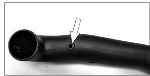
24. Install the provided grommet into the K&N® intake tube as shown.
