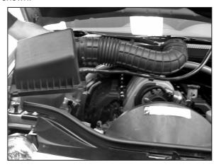
6. Remove the upper air box housing and intake tube assembly as shown.
