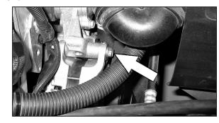
14. Remove the upper alternator mounting bolt as shown.
