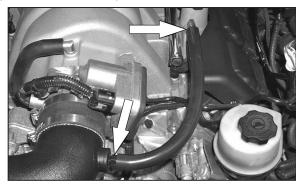
28. Install the provided crank case vent hose onto the valve cover fitting. Then, connect the open end to the 1/4" NPT fitting installed into the K&N® intake tube.
