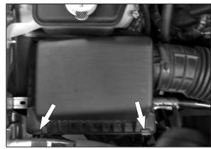
Release the two air box clam shell clips as shown.
