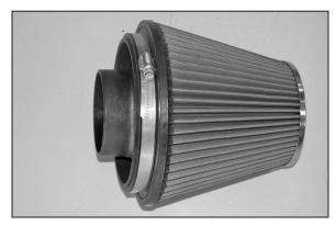
30. Install the air filter adapter into the K&N® air filter and secure with the provided hose clamp as shown.
