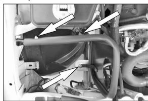
21. Install the heat shield assembly into the vehicle. Secure to the lower and upper air box mounts and washer bottle stud with the provided hardware.
