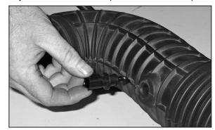
23. Remove the air temperature sensor from the stock intake tube as shown.
