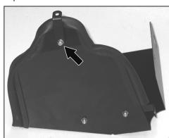
22. On 2007 model year vehicles, install the heat shield mounting bracket (#07805) to the side of the heat shield using the provided hardware.
