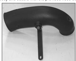
10. Install the tube mounting bracket (#06511) onto the K&N® intake tube (as shown) using the provided hardware.
