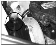
8. Remove the timing cover bolt (shown).
