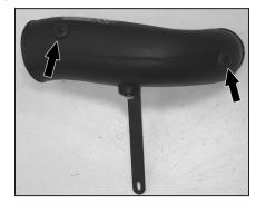
11. Install the provided grommets into the K&N<sup>®</sup> intake tube as shown.
