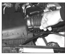
2. Disconnect the crank case vent hose from the air box lid as shown, then un-hook the crank case vent tube from the retaining clip.
