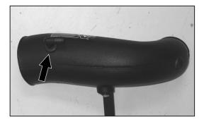
12. Install the provided 90° fitting into the grommet installed into the K&N® intake tube as shown.
