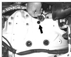
6. Remove the inner air box retaining grommet as shown.
