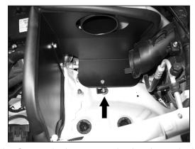
24. Secure the lower mounting bracket to the lower inner fender with the provided hardware.
