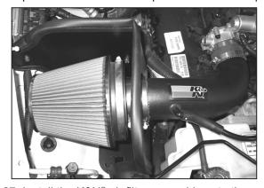
27. Install the K&N® air filter assembly onto the intake tube and secure with the provided hose clamp. Then connect the crank case vent line to the hose mender as shown and secure with the provided hose clamp.
