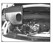
5. Pull up firmly on the air box assembly and remove it from the vehicle as shown.
