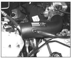
18. Connect the crank case vent hose to the 90° fitting installed into the K&N® intake tube as shown. NOTE: On 2011 and later vehicles use provided silicone hose.
