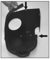
20. Install the provided edge trim onto the heat shield, starting at the bracket installed in step #19. NOTE: Some trimming of the edge trim may be necessary.
