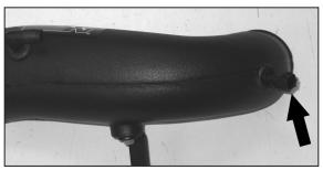
14. Install the air temperature sensor into the grommet installed in the K&N® intake tube as shown.
