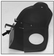
21. Install the heat shield mounting bracket (#070052) to the bottom of the heat shield using the provided hardware as shown.
