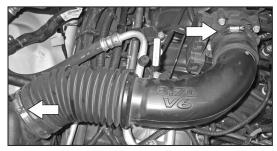
3. Loosen the two hose clamps which secure the stock intake tube to the throttle body and air box, then remove the intake tube from the vehicle.
