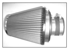
31. Install the provided silicone hose (08698) onto the filter assembly and secure with the provided hose clamp.
