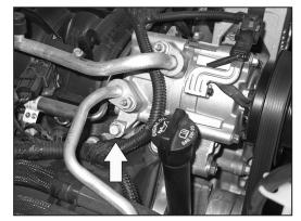
Remove the lower rear A/C compressor mounting bolt shown.
