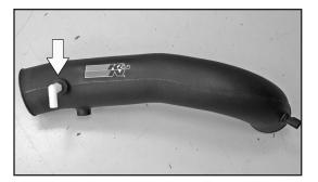
NOTE: Plastic NPT fittings are easy to cross thread. Install the vent fitting "hand" tight, then turn it two complete turns with a wrench.
