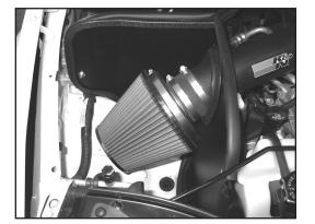
32. Install the filter assembly onto the intake tube and secure with the provided hose clamp.
