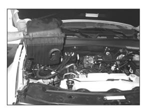
5. Lift up firmly to dislodge the air box from the mounting grommets and then remove the air box from the vehicle.
