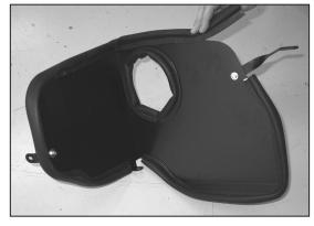
16. Install the provided edge trim onto the heat shield as shown.
