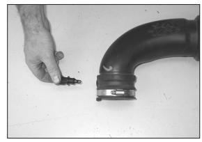
23. Remove the air temperature sensor from the factory intake tube as shown.
