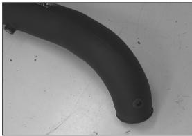
24. Install the supplied grommet into the intake tube as shown.
