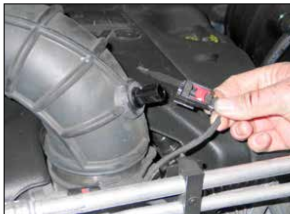
2. Release the red locking tab and then disconnect the inlet air temperature electrical connection.
