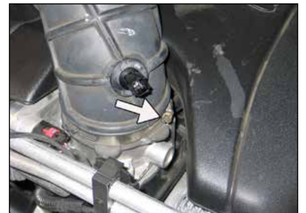
3. Loosen the hose clamp that secures the intake tube to the throttle body.
